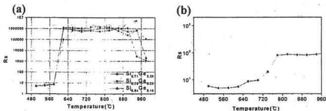
Fig. 1 Sheet resistance as a function of RTA temperature in  $N_2$  ambient for solid state reaction of Ni with (a)  $Si_{1-x}Ge_x$  ( $X=0.16, 0.25,$  and  $0.29$ ) and (b)  $X=0$ .
