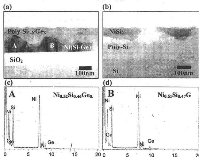
Fig. 5 (a) XTEM micrograph of  $Ni/Si_{0.75}Ge_{0.25}$ , (b)  $Ni/poly-Si$  after  $660^\circ C$  RTA, and (c), (d) corresponding EDS spectra.
