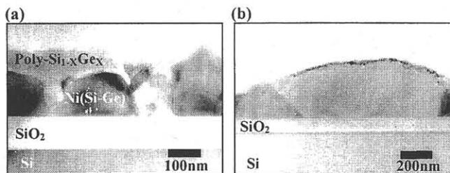
Fig. 6 XTEM micrograph of  $Ni/Si_{0.75}Ge_{0.25}$  (a) after  $580^\circ C$  RTA and (b) after  $900^\circ C$  RTA.
