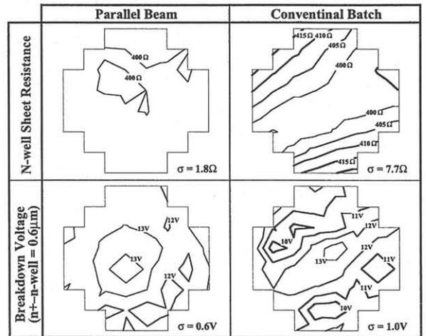
Fig. 7. Contour map of  $n$ -well sheet resistance and  $n^+/n$ -well breakdown voltage.
