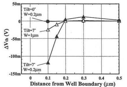
Fig. 9. Simulation on variation of threshold voltage for NMOSFET around well boundary.
