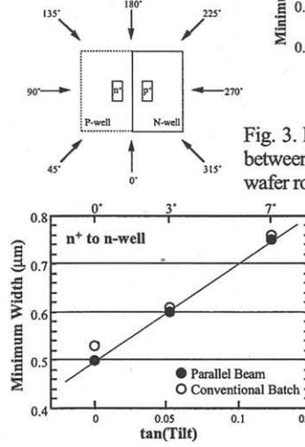
Fig. 6. Dependence of minimum spacing between  $n^+$  and  $n$ -well on tilt angle.
