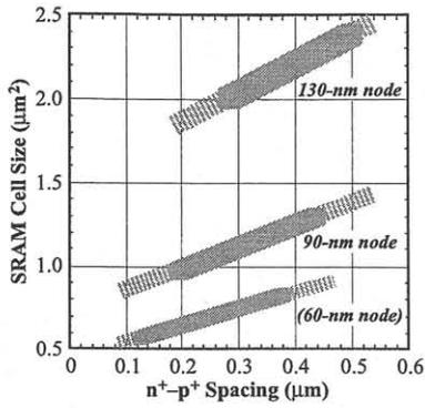
Fig. 1. Dependence of SRAM cell size on  $n^+ - p^+$  spacing.
