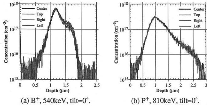
Fig. 5(a)-(b). SIMS profile of parallel beam.
