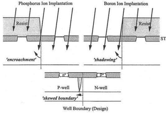
Fig. 2. Skew of well boundary caused by tilted implantation.
