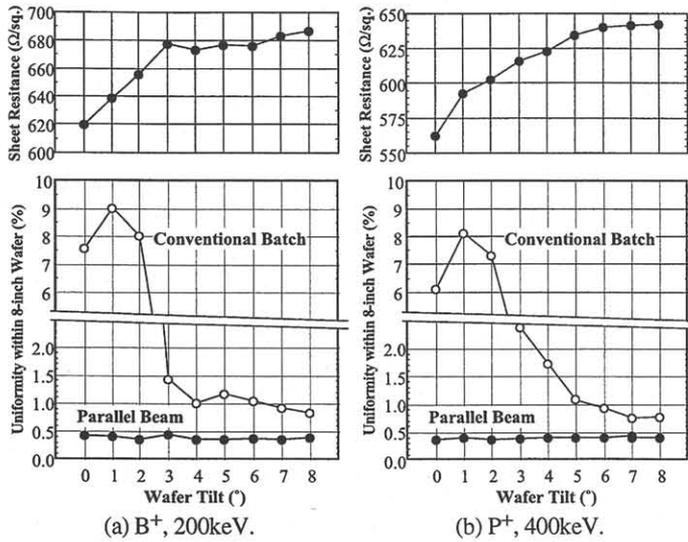
Fig. 4(a)-(b). Sheet resistance and its uniformity within 8-inch Wafer (after  $900^\circ\text{C}$  annealing).
