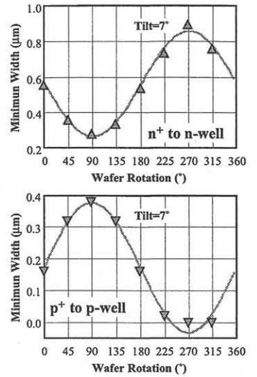
Fig. 3. Dependence of minimum spacing between well and source-drain diffusion on wafer rotation for  $7^\circ$ -tilted implantation.
