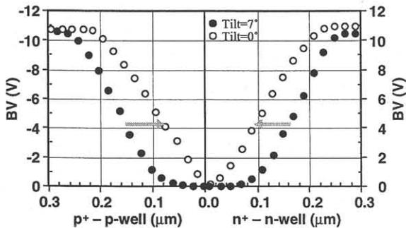
Fig. 8. Inter-well isolation using small tilt angle implantation by high-energy parallel beam.
