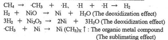
Fig. 2 Mechanism of the new treatment technique
