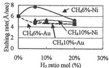
Fig. 3 Etching rate of Au and Ni
