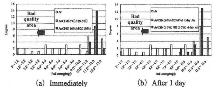
Fig. 5 Results measured the pull strength of wires on the samples
