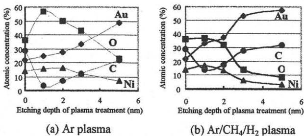
Fig. 4 Depth profile of each element in a Au pad
