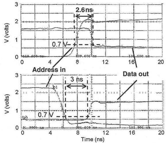
Fig. 4: Read "0" and Read "1" operations in a 1-kb FET array with the time interval from address change to data valid indicated.
