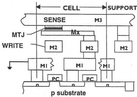
Fig. 2: 1 TJ-1 FET cell geometry
