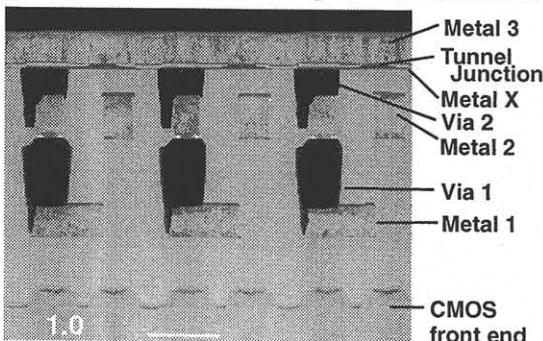
Fig. 3: TEM cross-section of three 1 TJ-1 FET cells.
