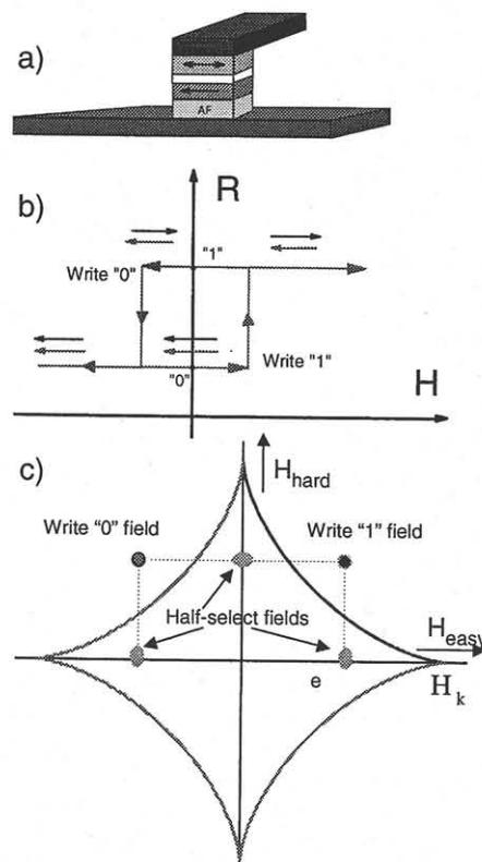
Fig. 1: Structure (a), resistance-magnetic field characteristic (b), and free layer stability boundary (c) of a magnetic tunnel junction.
