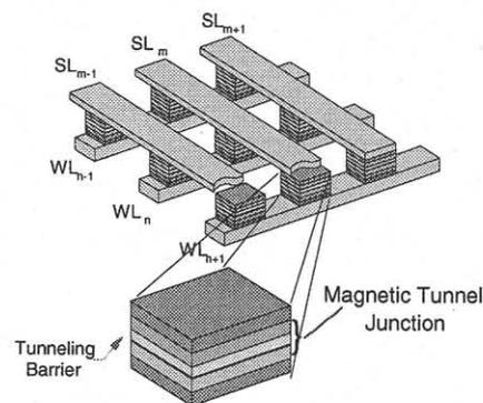
Fig. 5: Cross-point architecture
