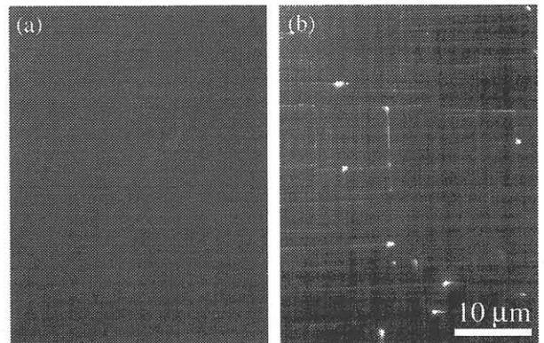
Fig. 6 Optical micrographs after defect etching for (a) the 30%-Ge sample and (b) a conventional graded SiGe virtual substrate
