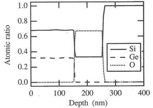
Fig. 4 Depth profiles for a 30%-Ge sample measured by RBS
