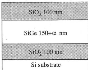
Fig. 2 Sample fabrication procedure
