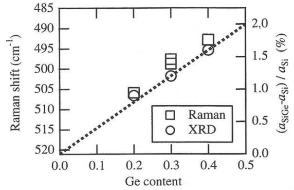
Fig. 3 Raman shift and lattice constant ratio as a function of Ge content in the SiGe layer
