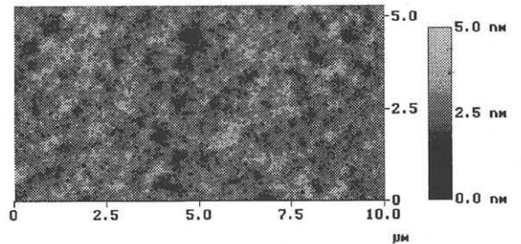
Fig. 5 AFM image of the 30%-Ge sample. The z-scale is 5 nm.
