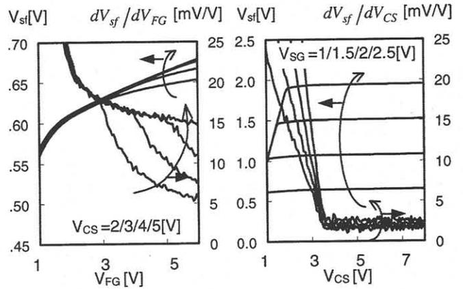
Fig. 7:  $V_{th}$  of  $M_{SG}$  monitored by  $V_{sf}$  for an accessible gate cell:  $V_{FG}$  sweep with  $V_{SG} = 1\text{V}$  (left) and  $V_{CS}$  sweep with  $V_{FG} = 4\text{V}$  (right).
