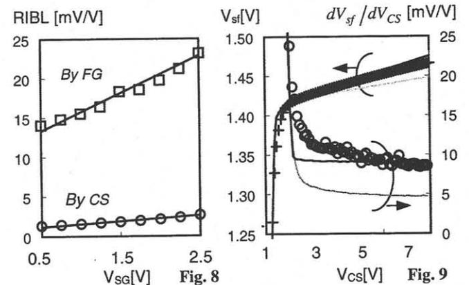
Fig. 8:  $V_{SG}$  dependence of RIBL at programming condition ( $V_{CS} = 5\text{V}$ ): measurement-symbol, approximation-line.
