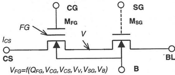
Fig. 2: Equivalent MACRO cell of SSI Flash cell.  $V$  represents a virtual node between the two transistors.  $V_{FG}$  is coupled by 5 capacitors between CG, CS, V, SG, B. Dotted line on  $M_{SG}$  is intended to represent the effect of remote electrodes on  $M_{SG}$ .
