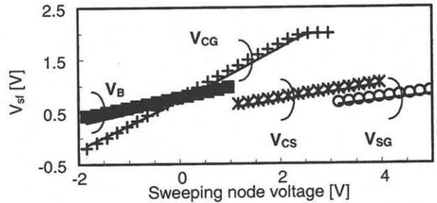
Fig. 6: Coupling of  $V_{FG}$ , represented here by  $V_{sf}$ , from other electrodes: measurement (symbols) and SPICE simulation (line).
