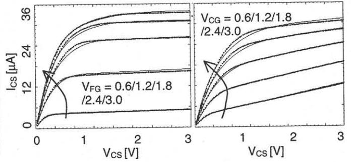
Fig. 5: I-V characteristics: measurement (solid line) and SPICE simulation (dotted line) for accessible gate cell (left) and for floating gate cell (right) at  $V_{BL} = V_B = 0$ ,  $V_{SG} = 1.2\text{V}$ .
