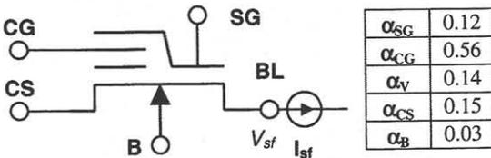
Fig. 4: Illustration of CR extraction technique and extracted CR's. Here  $V_{sf}$ , the voltage read at constant current source  $I_{sf}$ , is used to get  $V_{FG}$  by the relationship,  $V_{sf} = V_{FG} - V_{th}$  of  $M_{FG}$ . The CR's are extracted at "READ" condition and assumed to be constant.
