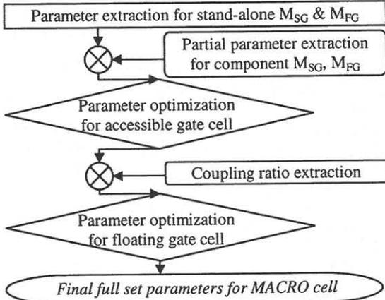
Fig. 3: Flow chart diagram for parameter extraction.
