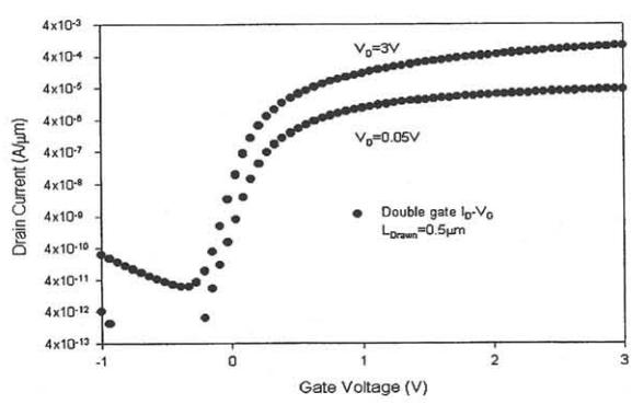
Fig.6. Subthreshold characteristics of a short channel double gate device
