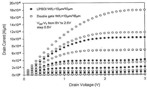
Fig.5. I-V characteristics of single and double gate LPSOI MOSFETs
