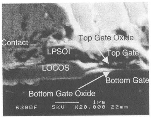
Fig.3. SEM picture of the proposed double gate device
