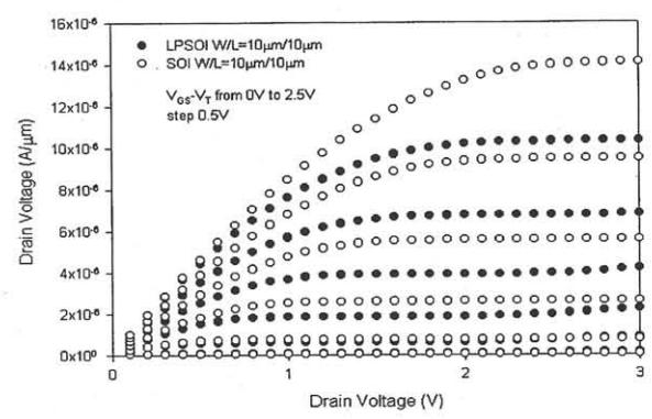
Fig.4. I-V characteristics of LPSOI and SOI MOSFET
