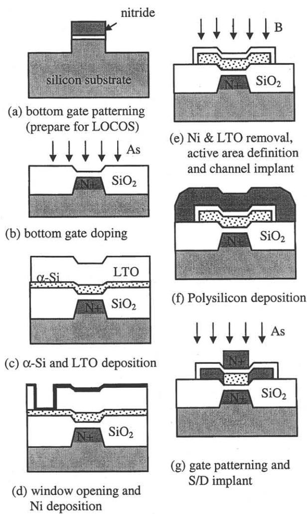
Fig.2. Fabrication process double gate devices
