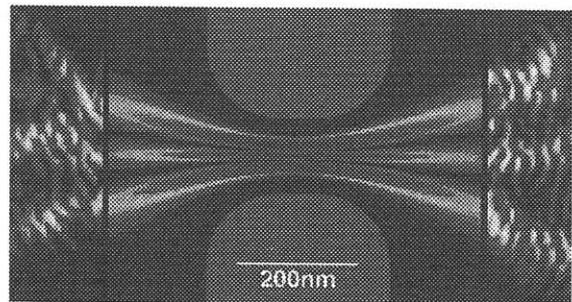
Fig. 2 SPM images of electron flow on the third conductance step, from the third mode of the QPC, with theory inside [1].
