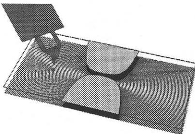
Fig. 1 Schematic diagram of the deflection of electron waves flowing from a quantum point contact with a charged SPM tip [2].
