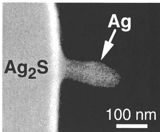
Fig. 4 The silver protrusion grown at the apex of the  $Ag_2S$  tip.
