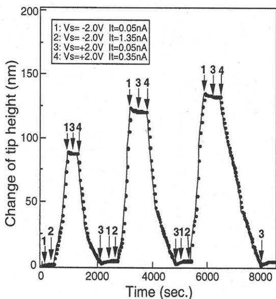
Fig. 3 Growth and shrinkage of the silver protrusion on the  $Ag_2S$  crystal. The  $Ag_2S$  crystal was used as a tip of a scanning tunneling microscope, and the change in the tip height was measured.
