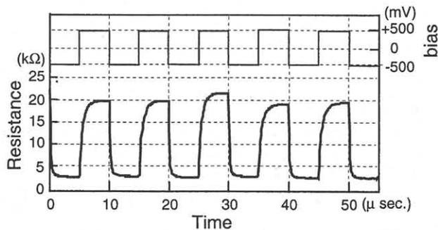
Fig. 6 Switching at 100 kHz.
