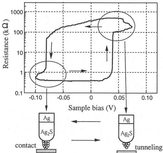
Fig. 5 Formation and deformation of a silver atomic bridge between the  $Ag_2S$  tip and the sample.
