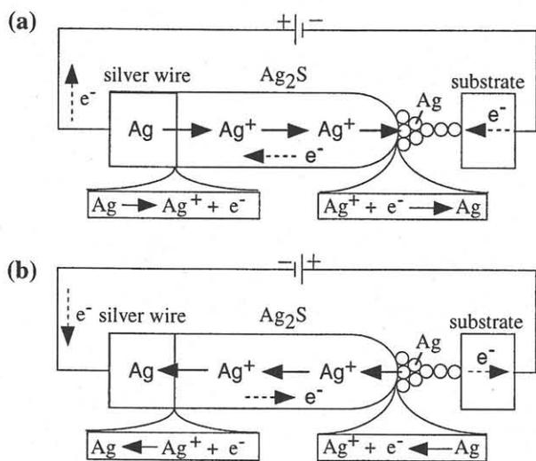
Fig. 1 Principle of a QPC switch. (a) Formation process, and (b) destruction process of the QPC.
