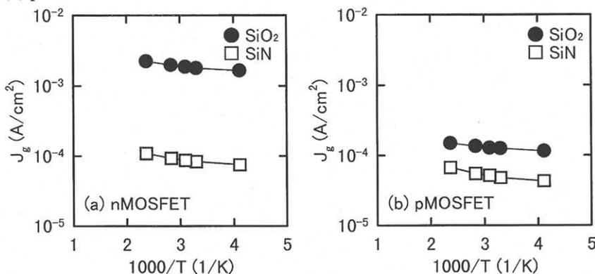
Fig.3 The temperature dependence of the gate leakage current. (a) nMOSFET and (b) pMOSFET.
