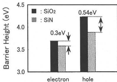
Fig.6 The barrier height of electron and hole.
