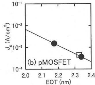
Fig.7 Calculation results of the direct tunneling. (a) nMOSFET and (b) pMOSFET.
