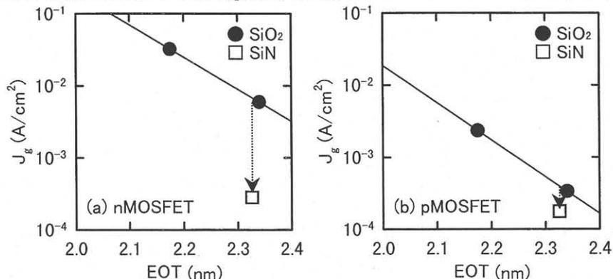
Fig.1 The relationship between EOT and the gate current of (a)nMOSFET and (b) pMOSFET.
