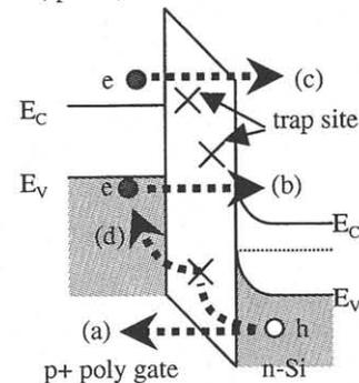
Fig.2 The possible conduction processes in pMOSFET.
