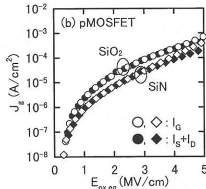
Fig.4 Carrier separation results of (a)nMOSFET and (b)pMOSFET.
