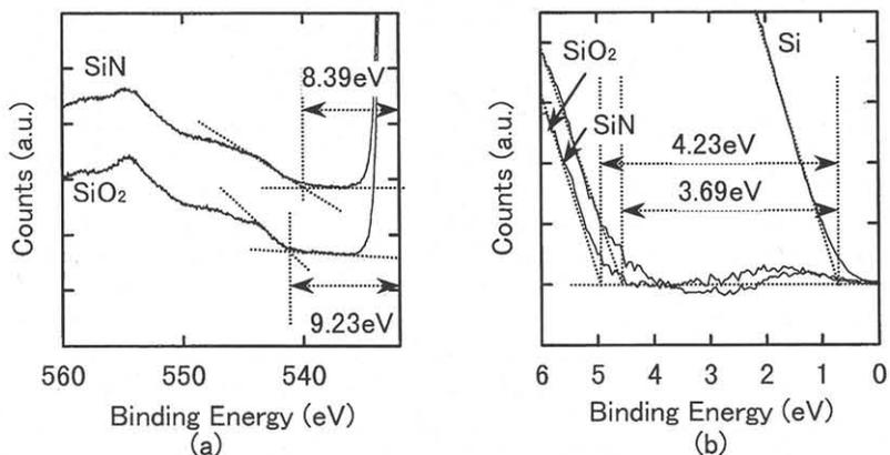
Fig.5 XPS spectrum of SiO<sub>2</sub>/Si and SiN/Si structures. (a) Energy loss spectrum of O1s. (b) Valence band spectrum.
