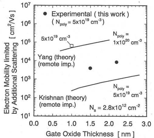
Fig.6 Mobility component of additional scattering term at  $N_s$  of  $2.8 \times 10^{12} \text{ cm}^{-3}$  as a function of  $T_{ox}$ . Solid lines show the calculated mobility by remote impurity scattering [1,2].
