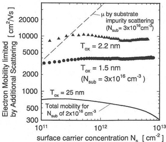
Fig.5 Mobility component of additional scattering mechanism, determined by Matthiessen's rule, as a function of  $N_s$ .
