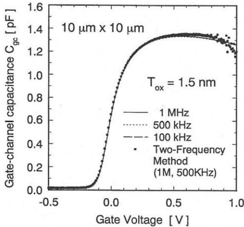
Fig.3  $C_{gc} - V_G$  characteristics of MOSFETs with  $L/W$  of 10  $\mu\text{m}/10 \mu\text{m}$  and  $T_{ox}$  of 1.5 nm.
