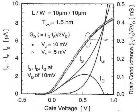
Fig.2 Drain, source and gate current (left axis) and drain conductance (right axis) as a function of  $V_G$ .
