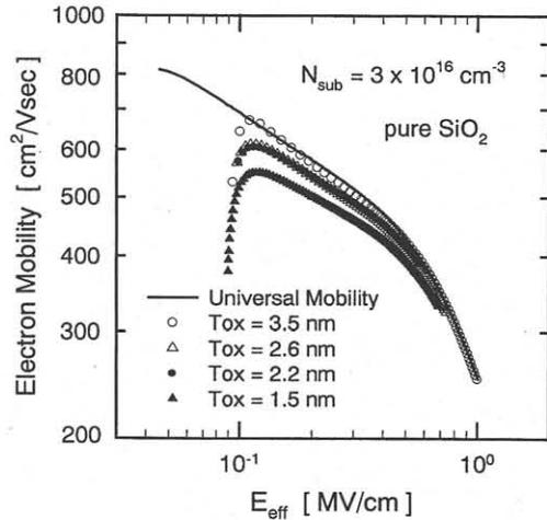
Fig.4 Inversion-layer electron mobility as a function of  $E_{eff}$  with  $T_{ox}$  of 3.5 - 1.5 nm. A solid line means the universal mobility
