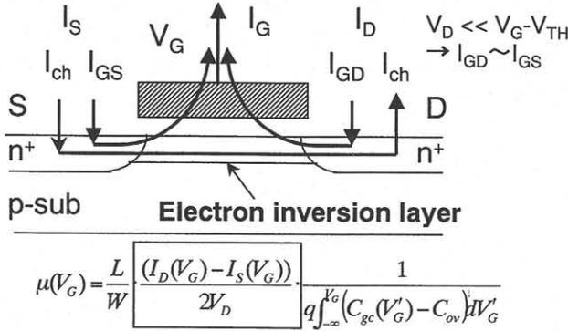
Fig.1 Schematic diagram of current flow of MOSFETs with high gate tunneling current. Here,  $I_s < 0$  and  $I_D > 0$ .
