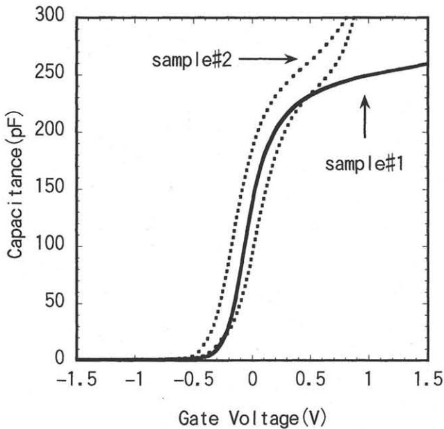
Fig. 2 High frequency capacitance-Voltage (C-V) curves for the  $\langle \text{Al/oxynitride/Si(100)} \rangle$  MOS structure. Notations are same in Fig. 1.
