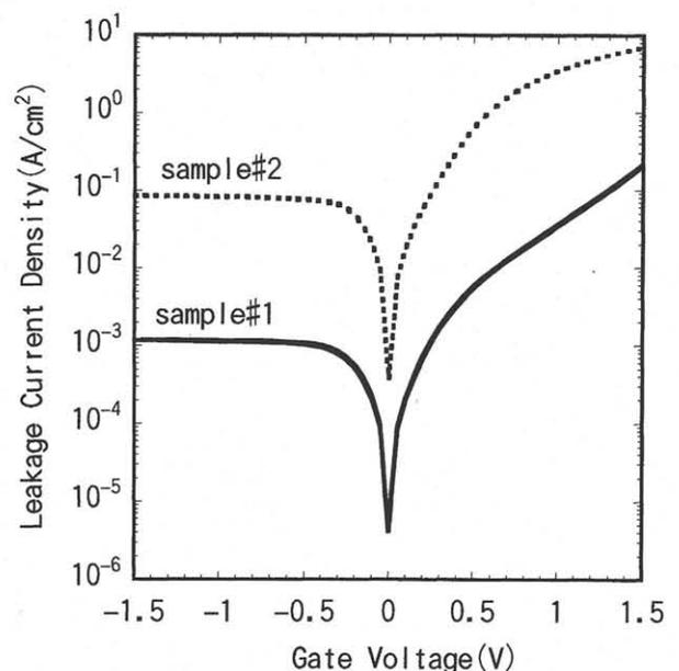
Fig. 1 Current-Voltage (I-V) curves for the <Al/oxynitride/Si(100)> structure: *sample #1* (oxynitride); *sample #2* (oxynitride with no chemical oxidation treatment).
