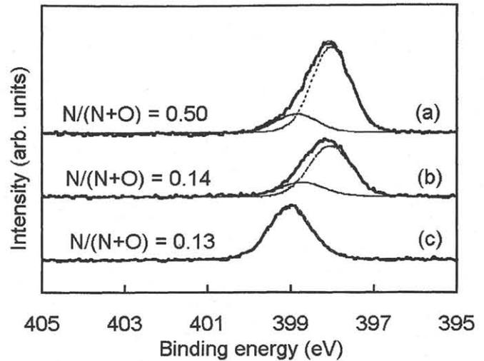
Fig. 3 N 1s energy region of XPS for *sample #1*: (a) as-nitrided; (b) after the chemical oxidation; (c) after the annealing of chemically oxidized specimen.
