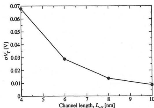
Fig.6: Standard deviation in threshold voltage,  $\sigma V_T$ , due to random discrete dopants in the source and drain of double gate MOSFETs with different channel lengths.
