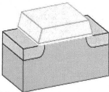
**Fig. 1** The current approach to semiconductor device simulation assumes continuous ionised dopant charge and smooth boundaries and interfaces.
