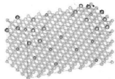
**Fig. 3** Sketch of a 4 nm MOSFET expected in mass production in 2020. There are less than 10 Si atoms along the channel. The size of the device becomes smaller than the size of biologically important molecules like ionic channels.
