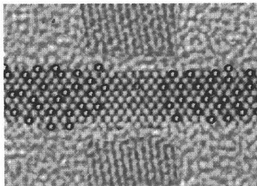
Fig.5: Impression of a 4 nm gate length double gate MOSFET illustrating the various sources of intrinsic parameter fluctuations.
