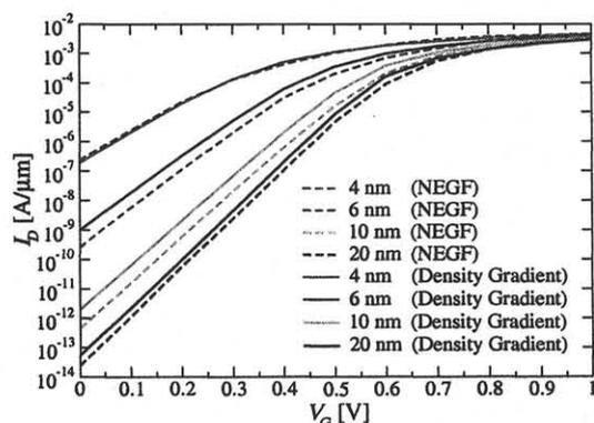
Fig. 4:  $I_D$ - $V_G$  characteristics obtained from non-equilibrium Green's functions simulations and calibrated DG simulations for double gate MOSFETs with gate lengths ranging from 20nm down to 4nm.  $V_D=1$  V and  $V_G$  applied to both top and bottom gate contacts.
