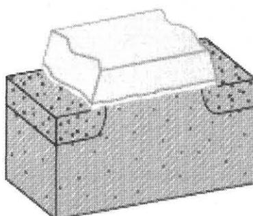
**Fig. 2** Sketch of a 20 nm MOSFET expected in mass production before 2010. There are less than 50 Si atoms along channel. Random discrete dopants, atomic scale interface roughness and line edge roughness introduce significant parameter fluctuations.
