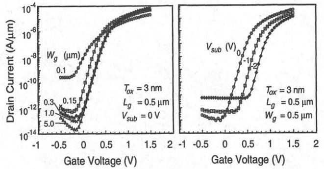
(a) Channel Width Dependence (b) Substrate Bias Dependence
