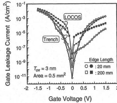
Fig. 6 Gate leakage currents of striped active regions for trench and conventional LOCOS isolation structures.
