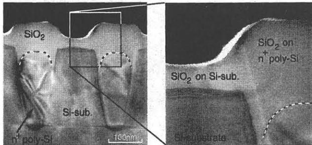
Fig. 4 TEM micrographs show conformal oxide formation along trench edges. Broken lines indicate oxidized polysilicon surfaces.
