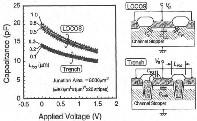
Fig. 8 Observed capacitances of multi-stripped  $n^+$ -junctions for the trench and LOCOS. Boron was implanted at 85 keV with a dose of  $9 \times 10^{12} \text{ cm}^{-2}$  after LOCOS formation and before trench etching.
