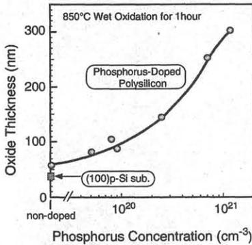
Fig. 3 Impurity Enhanced Oxidation (IEO) for 1 hour at 850°C in wet oxygen (40%  $\text{H}_2\text{O}$ ).
