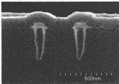
Fig. 2 SEM micrograph of obtained 0.1- $\mu\text{m}$  wide polysilicon shield trench isolation of which shoulders are covered with thick oxide.
