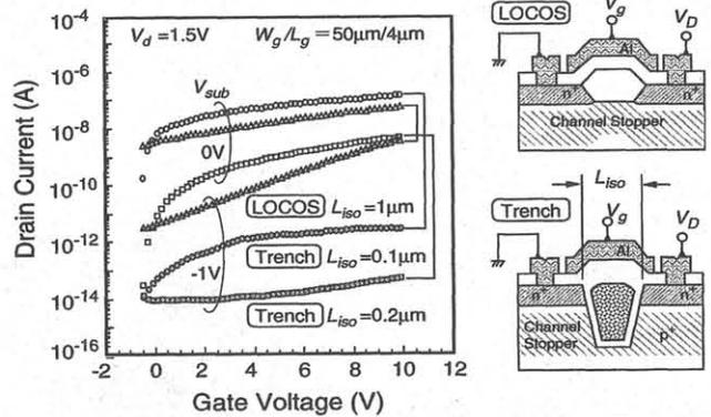
Fig. 7 Leakage currents between two adjacent  $n^+$ -junctions across isolation regions.
