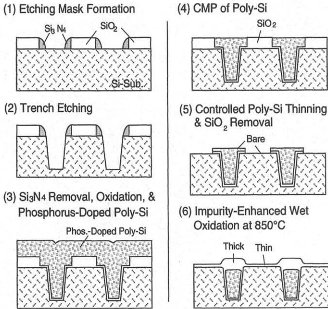
Fig. 1 A process sequence for proposed polysilicon-shield trench isolation utilizing impurity-enhanced oxidation.
