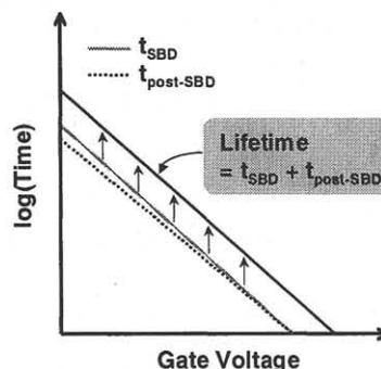
Fig. 7 Schematic illustration of the relation between the chip lifetime (i.e.  $t_{SBD} + t_{post-SBD}$ ) and  $V_g$  characteristics. The lifetime can be estimated from a parallel upward shift of  $\log(t_{SBD})$  vs.  $V_g$  characteristics.
