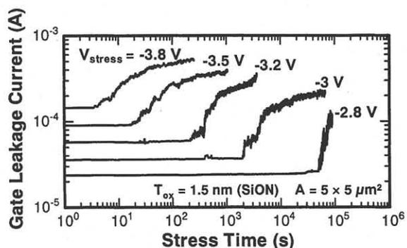
Fig. 2 Time evolution of gate current before and after SBD under various stress voltages. The degradation rate is slower for lower stress voltages.
