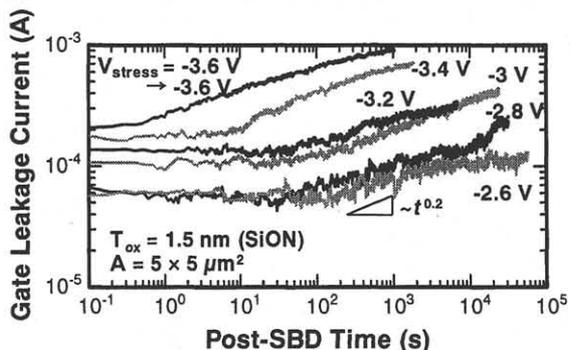
Fig. 4 Time evolution  $I_g$  during post-SBD degradation under various stress voltages. All SBD has been induced at  $V_g = -3.6$  V.
