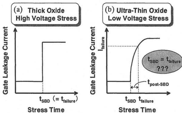
Fig. 1 Schematic illustration to compare the time evolution of gate current after SBD induced by (a) high and (b) low stress voltages.
