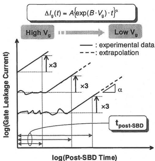
Fig. 5 Schematic illustration to show the post-SBD degradation.  $I$  versus  $t$  characteristics are well expressed by a power law.  $t_{post-SBD}$  is defined as a time for  $I_g$  to increase by a given factor from its initial value.
