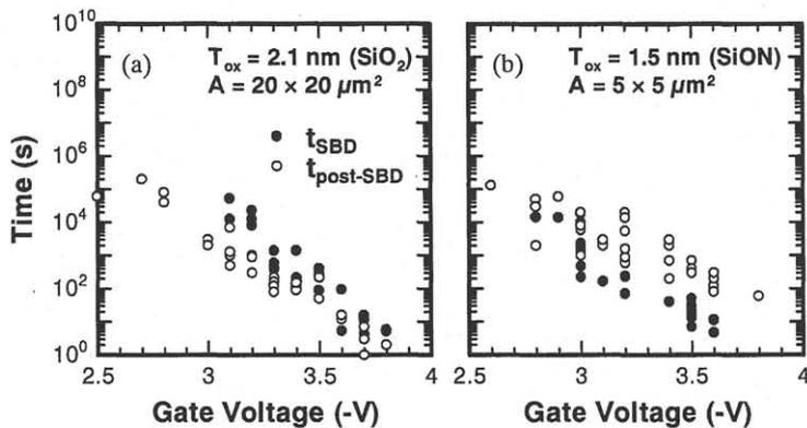
Fig. 6  $t_{SBD}$  and  $t_{post-SBD}$  for MOS capacitors with (a) 2.1 nm oxide and (b) 1.5 nm oxynitride are plotted as a function of stress voltage.
