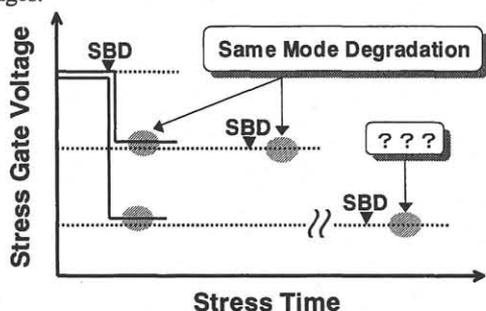
Fig. 3 Schematic drawing for the stress interruption technique (solid line) and the conventional CVS (dashed line). SBD is induced by using a high stress voltage, and then a low bias is applied to investigate the post-SBD degradation.
