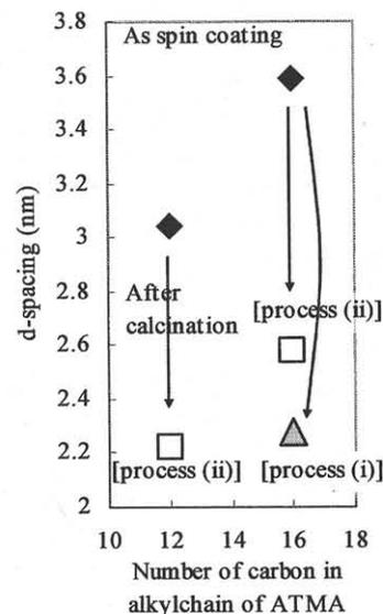
Fig.3 d-spacing of periodic porous silica film as a function of ATMA surfactant length
