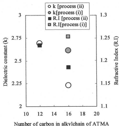
Fig.4 Dielectric constant and refractive index as a function of ATMA surfactant length
