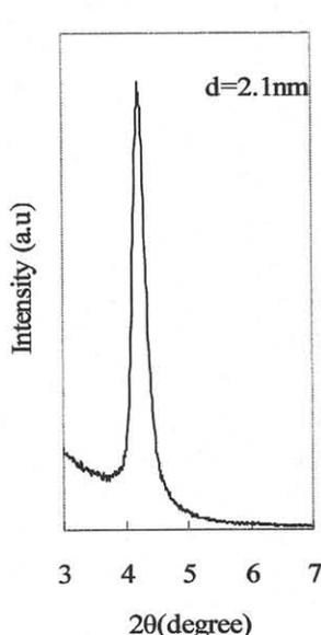
Fig.2 X-ray diffraction pattern for ordered porous silica film
