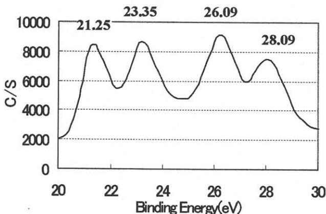
Fig.1 The XPS spectra of Ta4f of Ta film.
