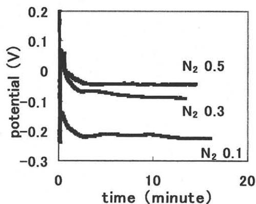
Fig.4 Time dependence of REDOX potential of various TaN film in the Cu electroless plating solution. 20°C. The REDOX potential of Cu is -0.01V.
