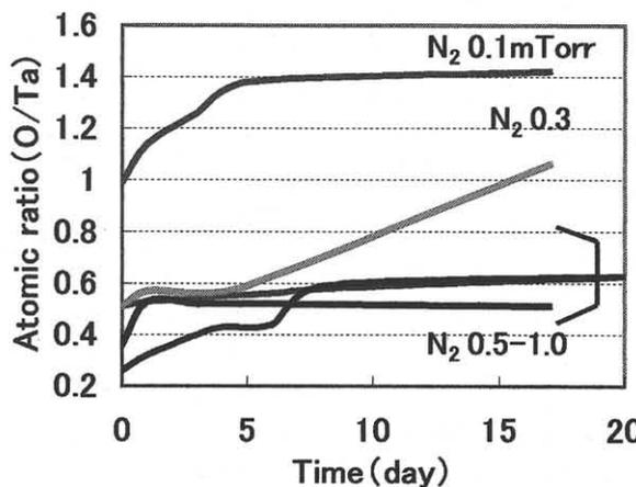
Fig.3 The atomic rate of O/Ta on the surface of TaN layers with time
