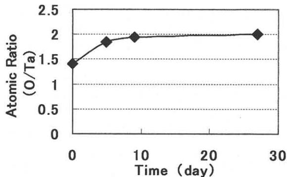
Fig.2 The atomic rate of O/Ta on the surface of Ta layer with time
