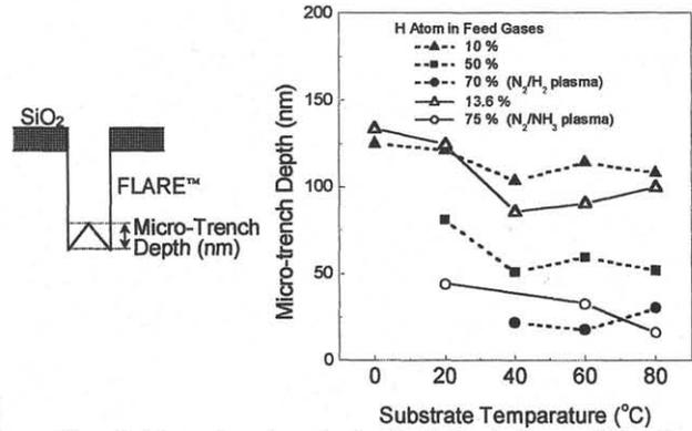
Fig. 6. The micro-trench depth at the bottom of the line shape as a function of the substrate temperature.
