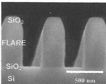
Fig. 4. SEM image of the etched profile of FLARE at UHF power of 1kW, N<sub>2</sub>/NH<sub>3</sub>=50/50 sccm and substrate temperature of 0°C.
