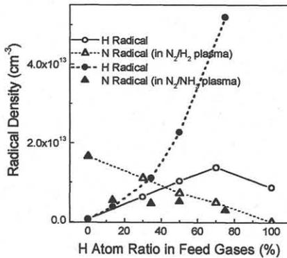
Fig. 3. N and H radical densities in UHF plasma measured using VUVAS technique as a function of H atom ratio in feed gases.
