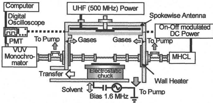
Fig. 1 Schematic diagram of UHF plasma etcher of 8 inch-wafer production level with the VUVAS system employing MHCL.
