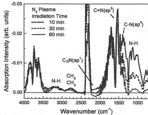
Fig. 7. The time evolution of absorption intensity spectra measured by FT-IR ATR when N<sub>2</sub> plasma was exposed to FLARE.
