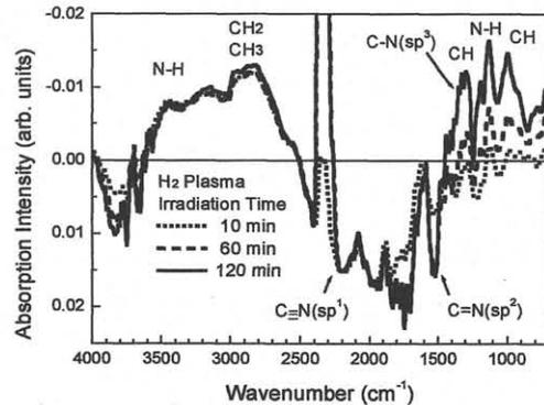
Fig. 8. The time evolution of absorption intensity spectra measured by FT-IR ATR when H<sub>2</sub> plasma was exposed to sample exposed by N<sub>2</sub> plasma.
