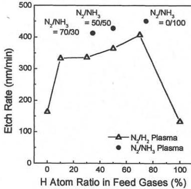
Fig. 2. The etching characteristics of FLARE™ using UHF-N<sub>2</sub>/H<sub>2</sub> and N<sub>2</sub>/NH<sub>3</sub> plasma as a function of H atom ratio in feed gases.
