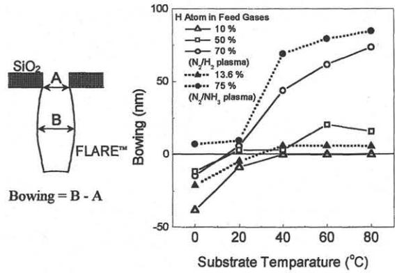
Fig. 5. The amount of bowing at sidewall of the line shape as a function of the substrate temperature.
