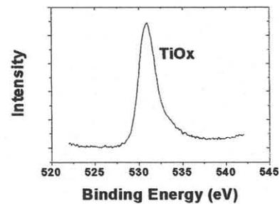
Fig. 5.  $O_{1s}$  XPS spectrum of Ti layer in Ru/Oxidation/PVD Ti/TiN structure
