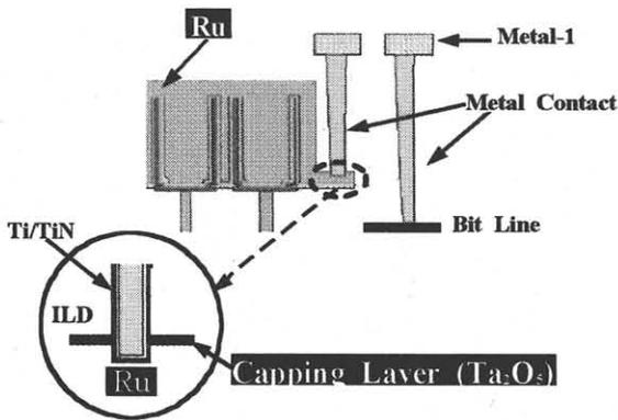
Fig. 1. Schematic cross section of the tested structure with RIS (Ruthenium Insulator Silicon) capacitor with  $Ta_2O_5$  capacitor and capping layer
