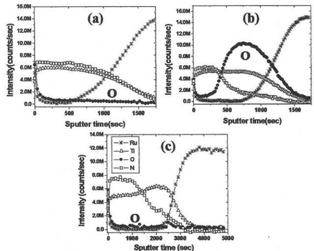
Fig. 6. AES depth profile of oxidized Ru/Ti/TiN stacks
