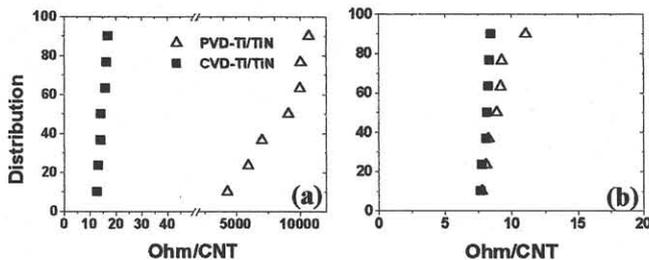
Fig. 2. Metal contact resistance (@  $0.2\mu m$ )
