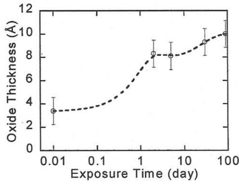
Fig. 2. Native oxide thickness on Si estimated by XPS, as a function of exposure time.
