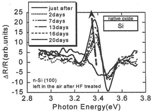
Fig. 1. PRS spectra as a parameter of exposure time in air.
