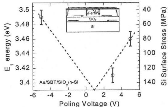
Fig. 5. Si surface stress in poled MFIS structure as a function of poling voltage..
