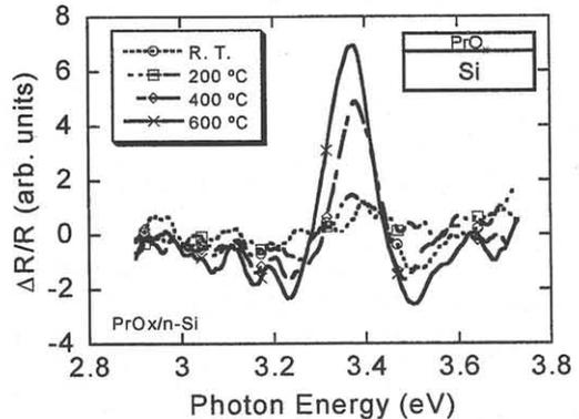
Fig. 4. PRS spectra of PrO<sub>x</sub>/Si deposited at different growth temperatures.
