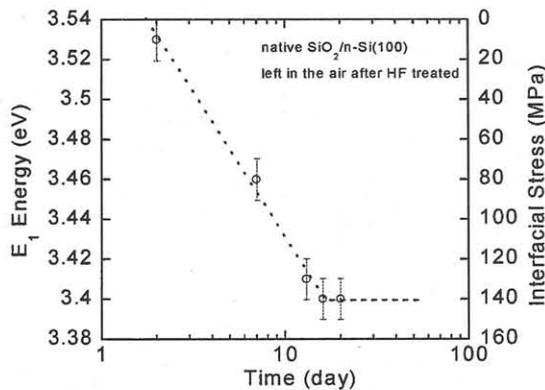
Fig. 3. Transition energy and Si surface stress in native oxide/Si as a function of exposure time.
