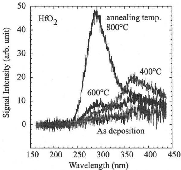
Fig. 1 Cathode luminescence spectra of HfO<sub>2</sub> films for as deposited sample (T<sub>s</sub> = 200°C) and T<sub>a</sub> = 400°C, 600°C, and 800°C samples.
