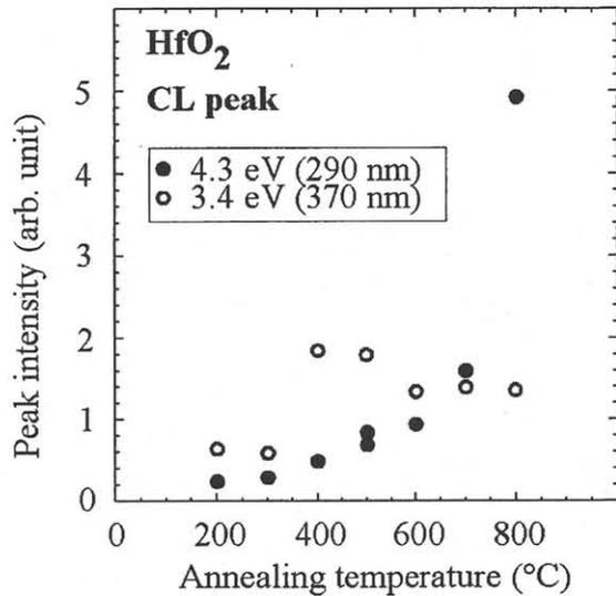
Fig. 2 CL peak intensity of two peaks at 4.3 eV and 3.9 eV as a function of annealing temperature.
