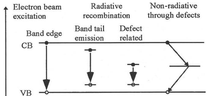
Fig. 3 Paths of electron-hole recombination.
