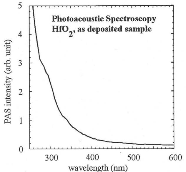
Fig. 4 Photoacoustic spectrum (PAS) of as-deposited HfO<sub>2</sub> film. The sample was deposited on a fused silica substrate.
