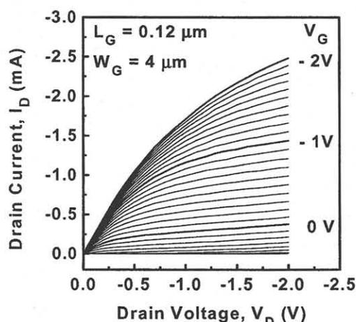
Fig. 2. Typical drain-current-voltage characteristics of 0.12- $\mu\text{m}$   $\text{Si}_{0.5}\text{Ge}_{0.5}$ -channel S<sup>3</sup>EMOSFET.
