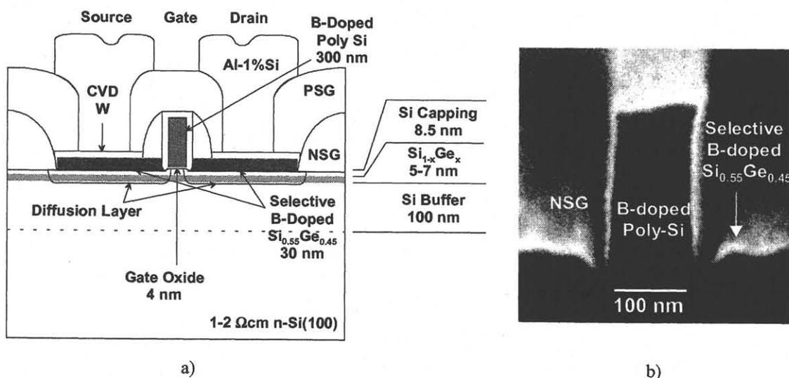
Fig. 1. a) Schematic diagram of  $\text{Si}_{1-x}\text{Ge}_x$ -channel super self-aligned ultrashallow junction electrode pMOSFET (S<sup>3</sup>EMOSFET) and b) the cross-sectional SEM micrograph of 0.12  $\mu\text{m}$   $\text{Si}_{0.5}\text{Ge}_{0.5}$ -channel S<sup>3</sup>EMOSFET
