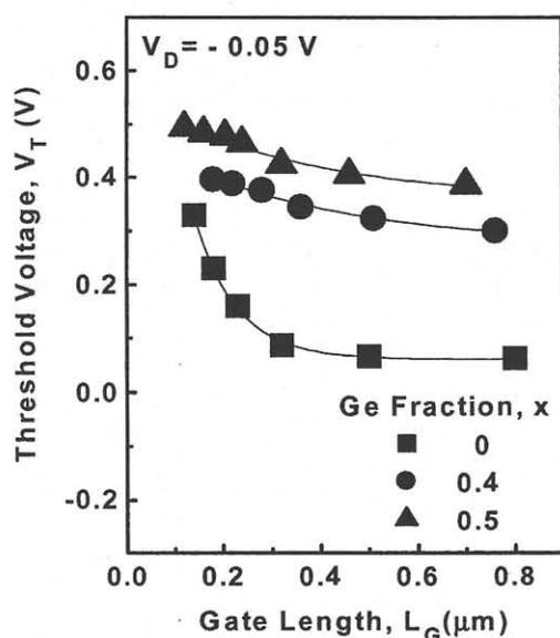
Fig. 3. Dependences of the threshold voltage when  $V_D = -50$  mV on the gate length of the  $\text{Si}_{1-x}\text{Ge}_x$ -channel S<sup>3</sup>EMOSFETs.
