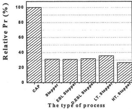
Figure 4. The variations of polarization values as a function of process
