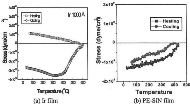
Figure 5. The variations of stress a function of temperature.
