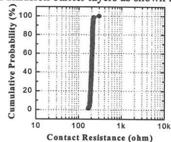
Figure 3. Distribution of BC contact resistance
