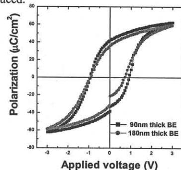
Figure 2. Hysteresis loops of 90nm and 180nm BE stack capacitors
