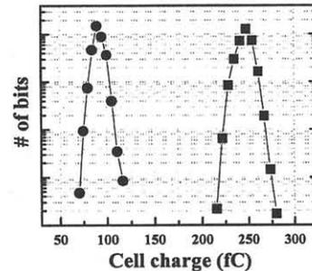
Figure 8. The measured charge distribution of 32Mb FRAM
