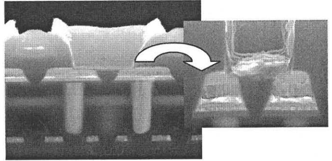
Figure 6. SEM image of fully processed 32Mb FRAM
