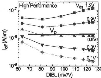
Fig.5. DIBL dependence of  $I_{off}$  in high performance devices. The critical drain voltage,  $V_o$ , can be defined. When  $V_{ds} < V_o$ , DIBL should be larger to suppress  $I_{off}$ . On the other hand, DIBL should be small when  $V_{ds} > V_o$ .
