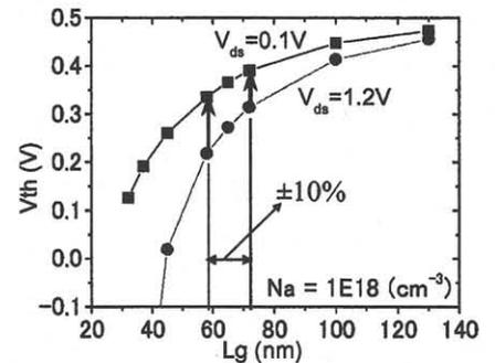
Fig.9.  $L_g$  dependence of  $V_{th}$  at  $V_{ds} = 1.2$  V and 0.1 V. The typical  $L_g$  is 65 nm and it is assumed that it varies in the range of  $\pm 10\%$ . The fluctuations of  $I_{off}$  can be suppressed in the present DIBL scheme because a device with worse short channel effect is more recovered
