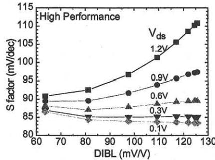
Fig.6. DIBL dependence of S factor in high performance devices. The S factor is improved when  $V_{ds}$  is reduced.
