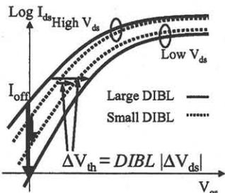
Fig.1. A Schematic of the DIBL effect. In a device with larger DIBL, off-current is more reduced when  $V_{ds}$  is low.
