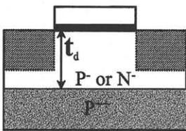
Fig.3. The device structure used in the simulation. An ideal step impurity profile is assumed.
