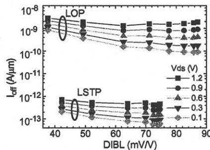
Fig.7. DIBL dependence of  $I_{off}$  in low power devices (LOP and LSTP).  $I_{off}$  decreases with increasing DIBL, because S factor degradation is not significant in low power devices (see Fig. 8).
