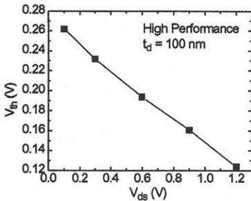
Fig.2. The typical  $V_{ds}$  dependence of  $V_{th}$ .
