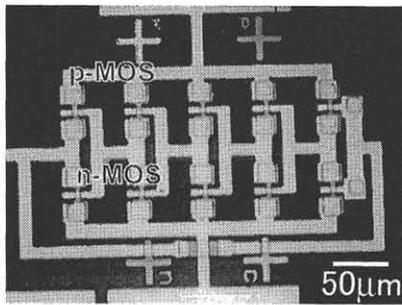
Fig. 4 Optical microscope view of a 5-stages CMOS ring oscillator.
