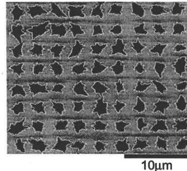
Fig. 2 SEM view of a Si film imprinted with a Ni-coated tip array and annealed at 590°C for 7 hours. The film was chemically delineated to remove a-Si region.
