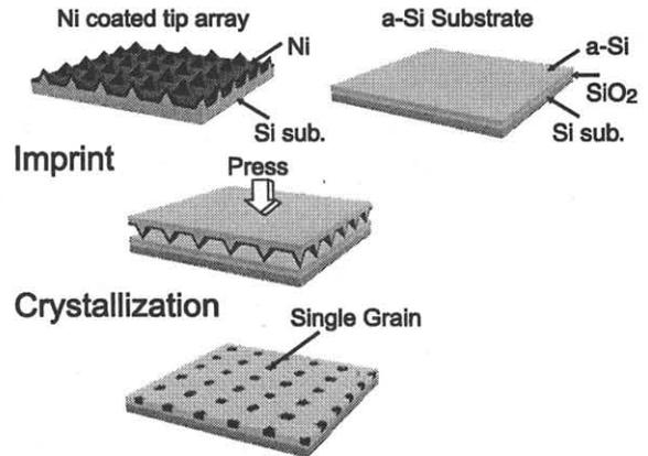
Fig. 1 Process sequence of the imprint technology. A tip-array is faced down and touched to the surface of an a-Si film. After removing the tip array, a-Si is annealed to crystallize.
