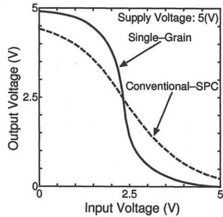
Fig. 5 Transfer characteristic of CMOS inverters fabricated with single-grain TFTs and with conventional-SPC TFTs.
