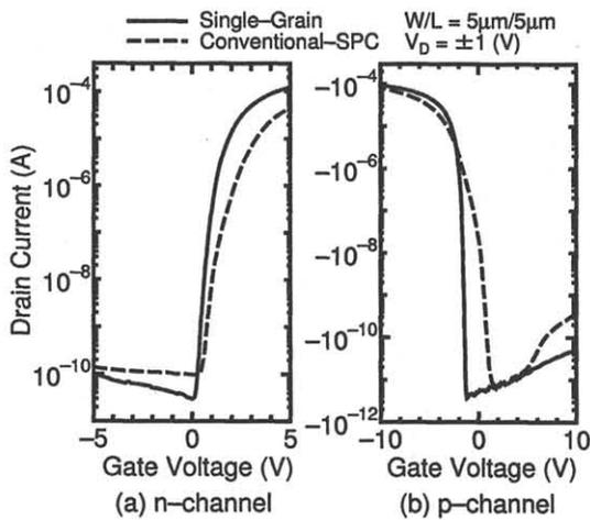
Fig. 3 Subthreshold characteristics of both (a) n-channel and (b) p-channel single-grain TFTs. Conventional-SPC TFTs are also shown.
