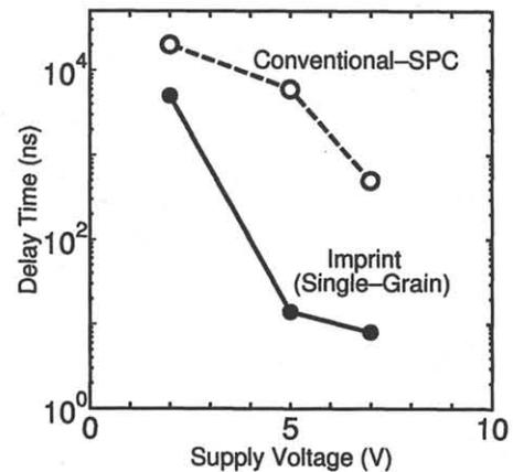
Fig. 6 Dependence of propagation delay time on supply voltage of 5-stages ring oscillator.
