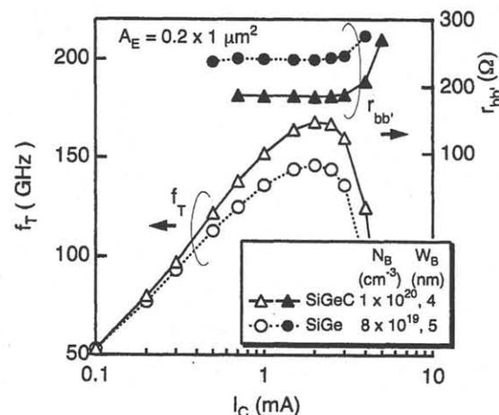
Fig. 6 Typical cutoff frequency and base resistance of a SiGe and SiGeC HBTs as a function of collector current.
