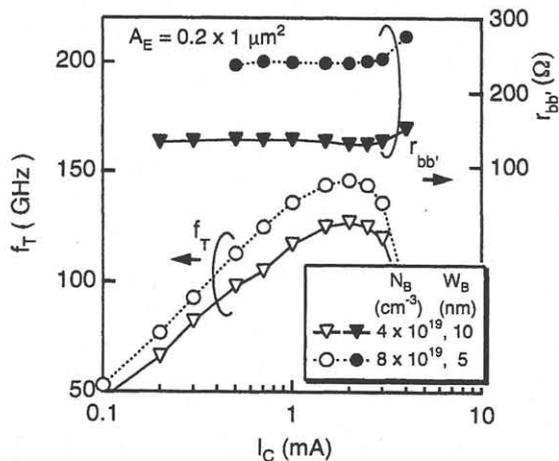
Fig. 5 Typical cutoff frequency and base resistance of SiGe HBTs as a function of collector current.
