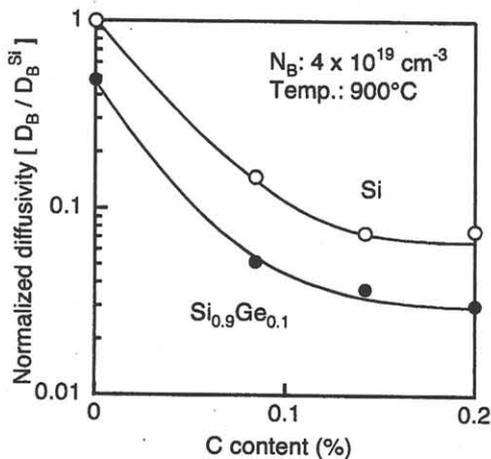
Fig. 1 Normalized B diffusivity in SiGeC layer as a function of C content.
