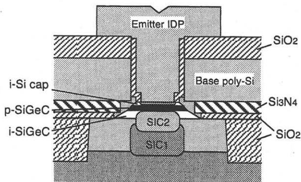
Fig. 3 Schematic cross-section of a SiGeC HBT.
