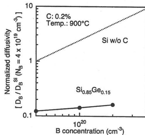
Fig. 2 Normalized B diffusivity in SiGeC HBT as a function of B concentration. Dotted line indicates B diffusivity in Si without C incorporation [6].
