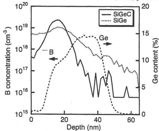
Fig. 4 SIMS profiles of B in SiGe and SiGeC HBTs.
