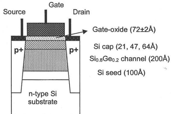
Fig. 1 Schematic cross-sectional view of the SiGe pMOSFET.
