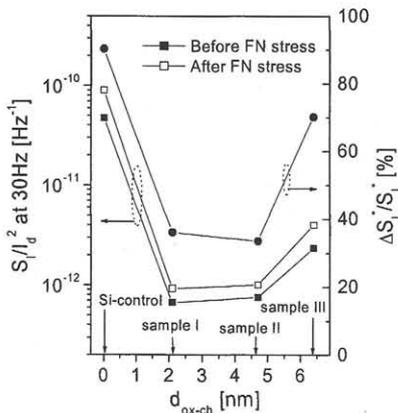
Fig. 3 Dependence of the 1/f noise at 30Hz on  $d_{\text{ox-ch}}$  before and after the F-N stress. The % change in  $S_f/I_d^2$  at 30Hz ( $\Delta S_f/I_d^2$ ) due to the F-N stress is also shown.
