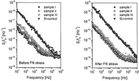
Fig. 2  $S_f/I_d^2$  vs. frequency for the SiGe pMOSFETs and the Si-control (a) before and (b) after the F-N stress measured at  $V_{\text{ds}}=100\pm 5\text{mV}$  and  $V_{\text{g}}=V_{\text{th}}-0.7\text{V}$ .
