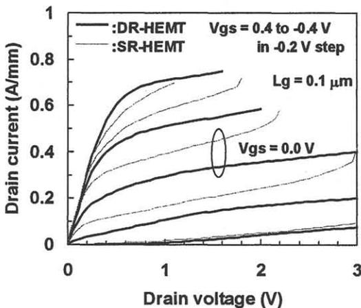
Fig. 3 Typical I-V characteristics for DR- and SR-HEMTs
