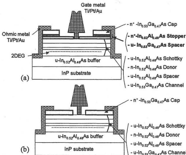
Fig. 1 Schematic cross-sections of the (a) DR- and (b) SR-HEMTs
