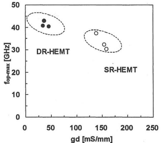
Fig. 4 Dependence of maximum operation frequencies of static 1/2 frequency divider ICs on  $g_d$  for DR- and SR-HEMTs
