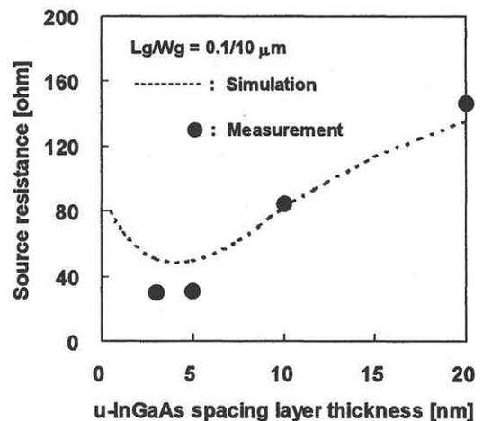
Fig. 2 Dependence of  $R_s$  on u-InGaAs spacing layer thickness
