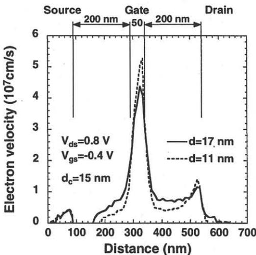
Fig. 4 Electron-velocity profiles in the InGaAs channel of 50-nm-gate lattice-matched HEMTs with  $d = 11$  and  $d = 17$  nm calculated by using MC simulations.
