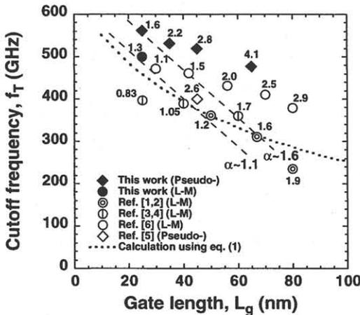
Fig. 3 Gate length  $L_g$  dependence of the cutoff frequency  $f_T$  in our present and previous works [1-6].
