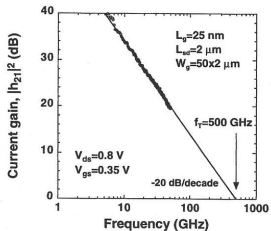
Fig. 1 Frequency dependence of the current gain  $|h_{21}|^2$  for a 25-nm-gate lattice-matched HEMT.
