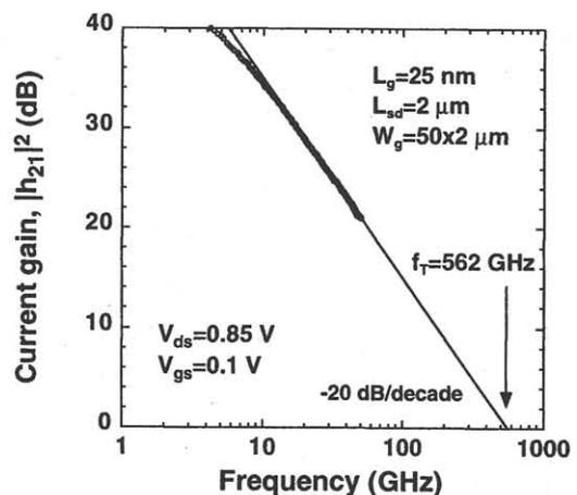
Fig. 2 Frequency dependence of the current gain  $|h_{21}|^2$  for a 25-nm-gate pseudomorphic HEMT.
