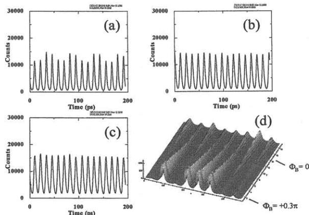
Fig. 3 All-optical regeneration at 84 Gb/s. (a) Input random pulses, (b) local clock pulses, (c) output random pulses, and (d) waveforms as a function of the interferometer phase bias.
