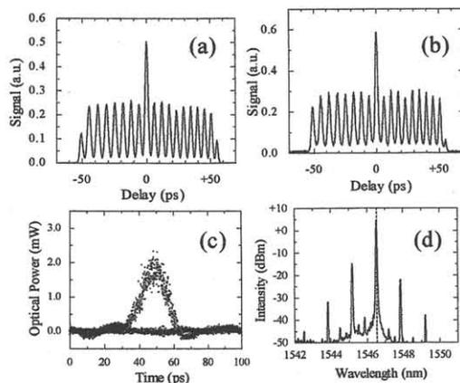
Fig. 4 Wavelength conversion at 168 Gb/s. Autocorrelation trace for the input random pulses (a), that of the output random pulses
