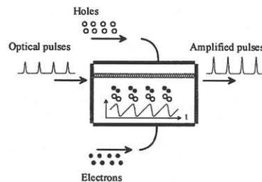
Fig. 2 Nonlinear refractive-index changes are induced by stimulated amplification in the SOA's.
