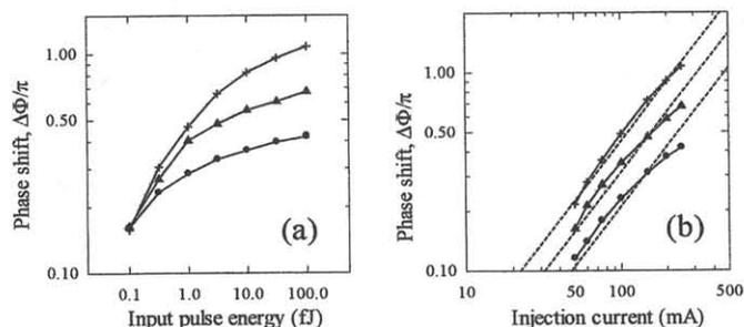
Fig. 5 Measured nonlinear phase shifts as functions of the input pulse energy and the injection current to the SOA. The input pulse frequencies were 168 GHz (circles), 84 GHz (triangles), and 42 GHz (crosses).
