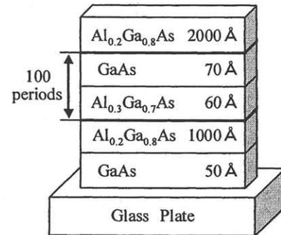
Fig.1 Structure of designed PRQW device
