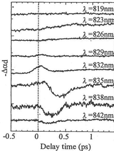
Fig.3 Differential transmission transients for various wavelengths
