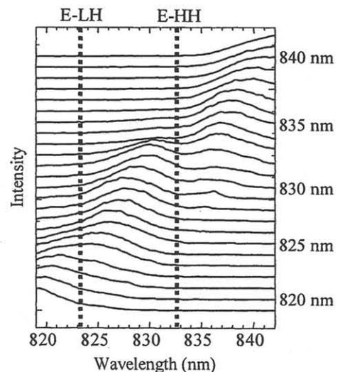
Fig.2 Transmission spectra for different central wavelengths of 100-fs pulses
