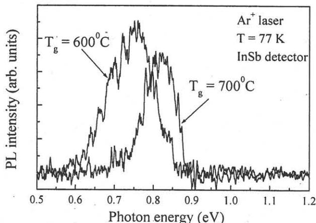
Fig.2 PL spectra of multilayer structures with islands (five periods) grown at  $T_g=600^\circ\text{C}$  and  $T_g=700^\circ\text{C}$ . The measurements were carried out at 77 K by InSb detector.
