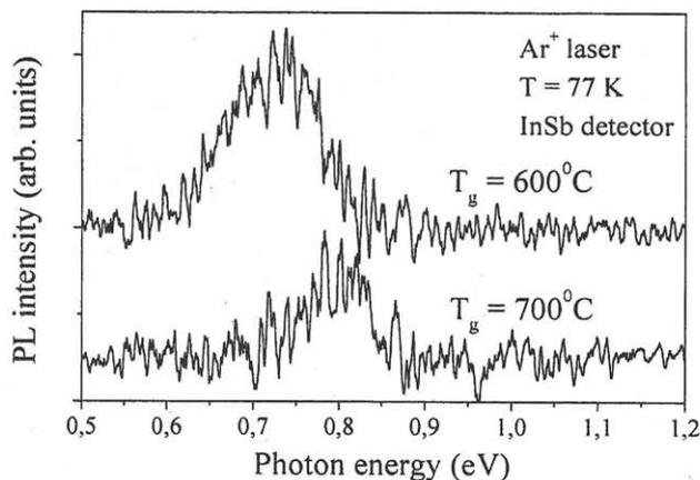
Fig.1 PL spectra of structures with islands grown at  $T_g=600^\circ\text{C}$  and  $T_g=700^\circ\text{C}$ . The measurements were carried out at 77 K by InSb detector.
