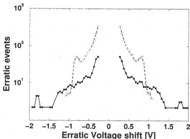
Fig. 5. Distribution of PE (solid line) and EE (dashed line) erratic threshold voltage shifts.
