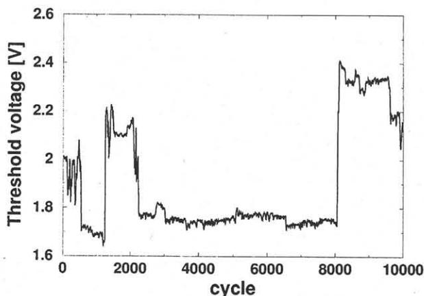
Fig. 1. Example of an erratic cell featuring both negative and positive jumps during cycling.
