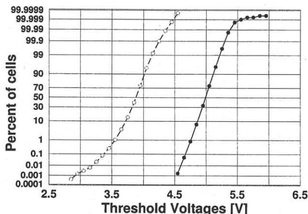
Fig. 2. Distributions of erased (dashed line) and programmed (solid line) thresholds.
