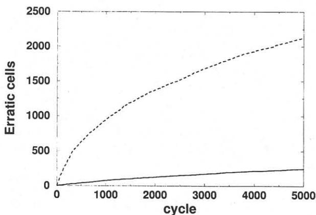
Fig. 4. Cumulative number of erratic bits during programming (PE - solid line) and erasing (EE - dashed line).
