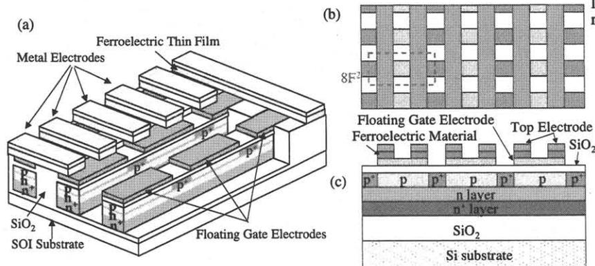
Fig. 5. A proposed planar  $8F^2$  cell array. (a) 3 dimensional view, (b) top view and (c) cross section along with a Si stripe.
