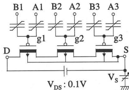
Fig. 7. Schematic of simulated circuit of a  $1 \times 3$  array.
