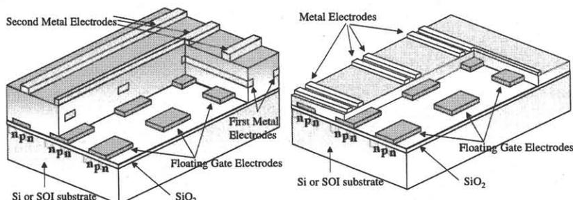
Fig. 2. A 1T2C-type ferroelectric memory array.
