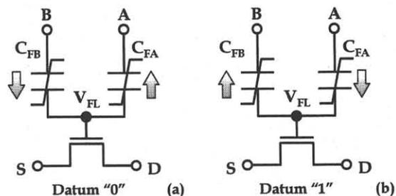
Fig. 1. 1T2C-type ferroelectric memory cell.
