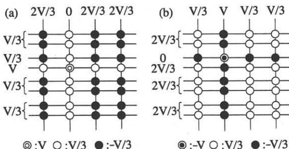
Fig. 4. "Write" operation for a proposed novel array structure. To complete the operation, the first (a) and second (b) pulses are applied successively. Vertical and horizontal lines represent Si stripes and top electrodes of ferroelectric capacitor, respectively.
