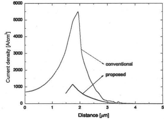
Fig. 5 Current density underneath n+ source during UIS.
