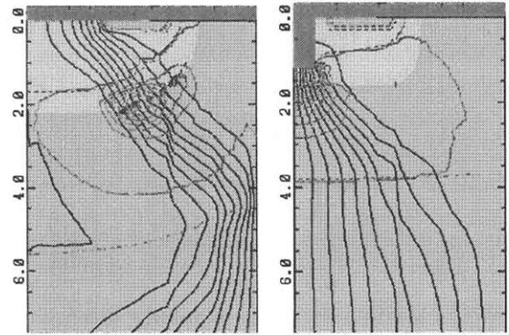
Fig. 4 Current flow and impact ionization at UIS.
