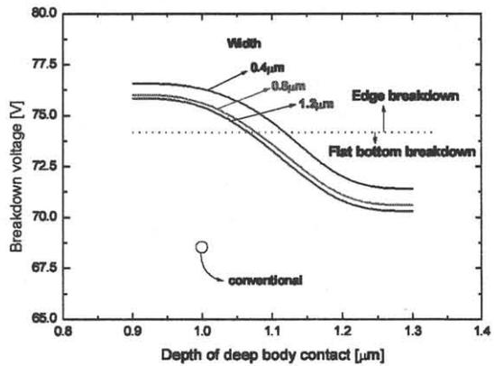
Fig. 6 Optimization of width and depth of deep body contact.
