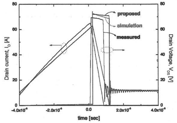
Fig. 3 Waveforms during the UIS.
