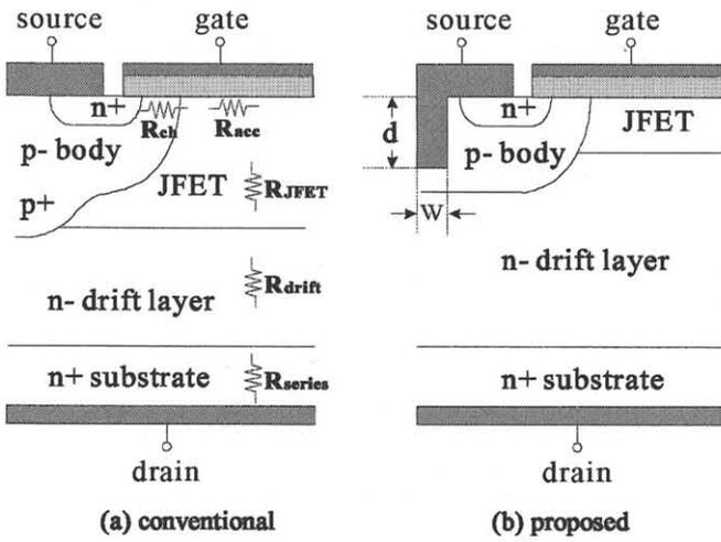
Fig. 1 Cross-sectional View
