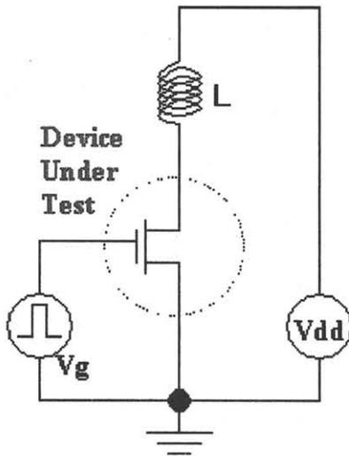
Fig. 2 Circuit diagram of UIS.
