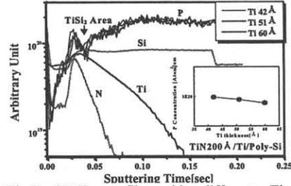
Fig.3 SIMS profile with different Ti thicknesses of TiN/Ti/poly-Si area in cell region after RTA 845°C.
