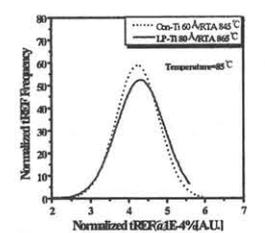
Fig.12 Frequency distribution of normalized data retention [tREF@1E-4% failure rate] in memory cells.
