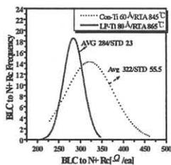
Fig.9 Frequency distribution of BLC to n+ Rc area in wafer for splitting conditions.
