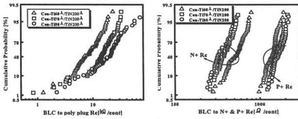
Fig.2 Cumulative probability of BLC to poly plug Rc in cell region and BLC to N+ Rc & P+ Rc in periphery area for each splitting condition in Group-1.
