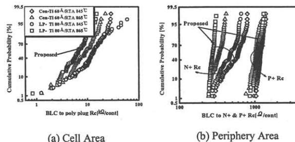
Fig.6 Cumulative probability of BLC to poly plug Rc in cell region and BLC to N+ & P+ Rc in periphery region to obtain the effect of Ti deposition condition and subsequent RTA in Group-2.
