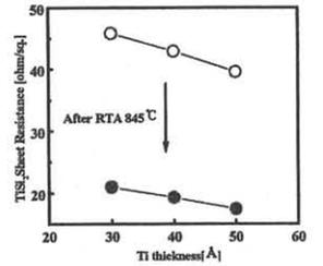
Fig.4 TiSi<sub>2</sub> sheet resistance [Rs] characteristics with different Ti thicknesses in BLC to n+ Rc area.
