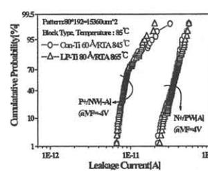
Fig.10 Comparison of N+/PW and P+/NW junction leakage in each wafer.
