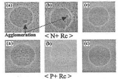
Fig.7 SEM image of Ti deposition condition with subsequent RTA. (a) Con-Ti 60 Å / 845°C, (b) LP-Ti 80 Å / 845°C and (c) LP-Ti 80 Å / 865°C
