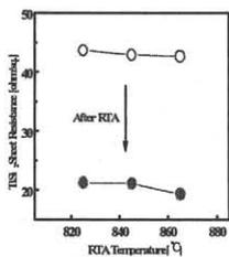
Fig.8 Sheet resistance of TiSi<sub>2</sub> with subsequent RTA temperatures in BLC to n+ Rc area.
