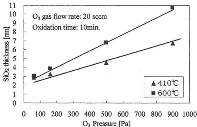
Fig. 3 O<sub>3</sub> pressure dependence of Si oxidation rate.
