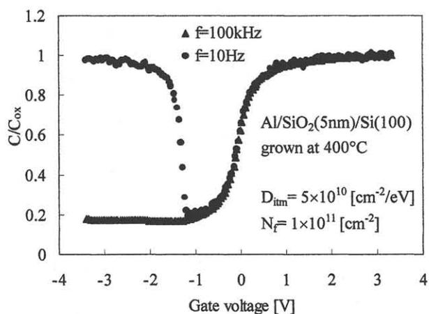
Fig. 4 High-frequency and quasi-static C-V curves of O<sub>3</sub> oxides.
