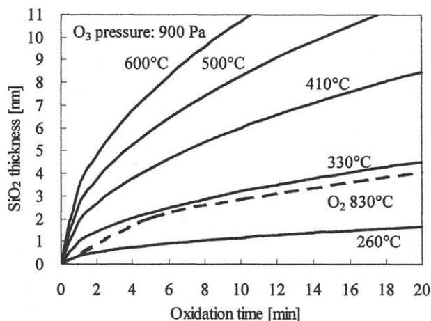
Fig. 2 Oxidation rate of hydrogen-terminated n-Si(100).
