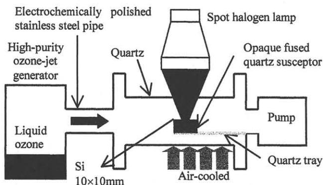
Fig. 1 Schematic view of the 100% O<sub>3</sub> oxidation system.
