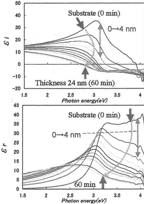
Fig. 2: Real part ( $\epsilon_r$ ) and imaginary part ( $\epsilon_i$ ) of the pseudodielectric function spectra obtained by ellipsometry measurement during deposition of  $Y_2O_3$  films. Substrate temperature  $T_s = 500^\circ C$ .
