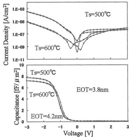
Fig. 5: I-V and C-V characteristics of  $Y_2O_3$  films with  $T_s = 500^\circ C$  and  $600^\circ C$ .
