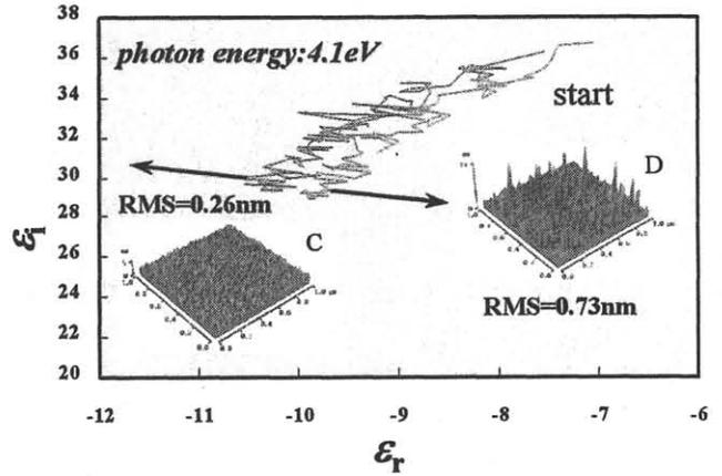
Fig. 3: Trajectories of ellipsometry signal in the plane of  $\epsilon_r$  and  $\epsilon_i$  from start to about 3nm-thick  $Y_2O_3$  film deposition. AFM images of each film are also shown.  $T_s = 560^\circ C$ .
