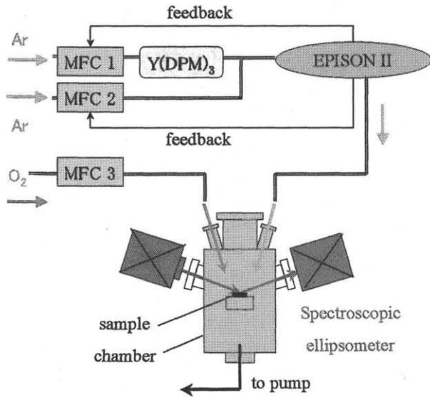
Fig.1: A schematic diagram of the present MOCVD system.
