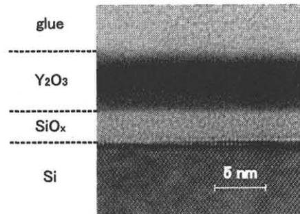
Fig. 4: Cross-sectional TEM image of a 8 nm-thick  $Y_2O_3$  film.  $T_s = 600^\circ C$ .
