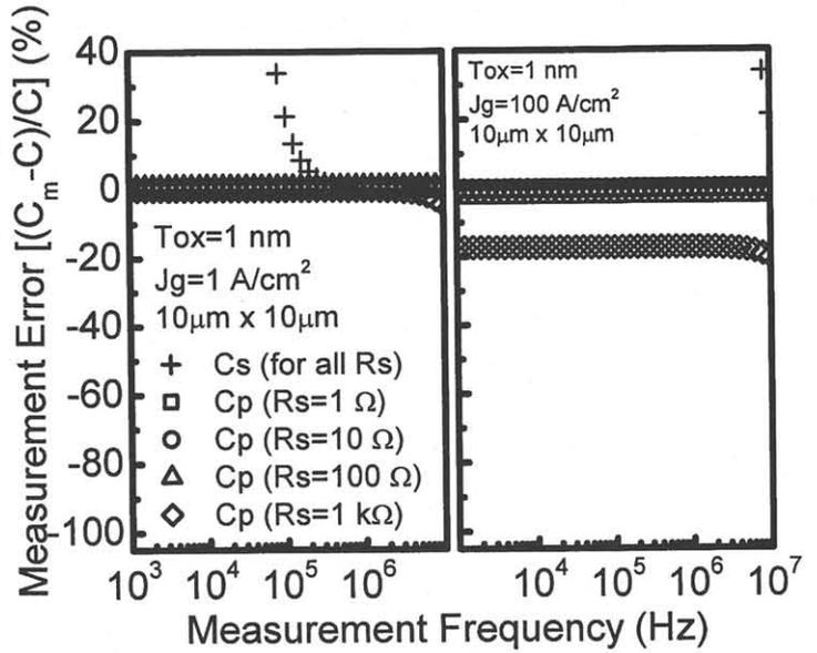
Fig. 4 Systematic error is reduced for smaller device area, consistent with [2]. The series (spreading) resistance does not scale linearly with device area.
