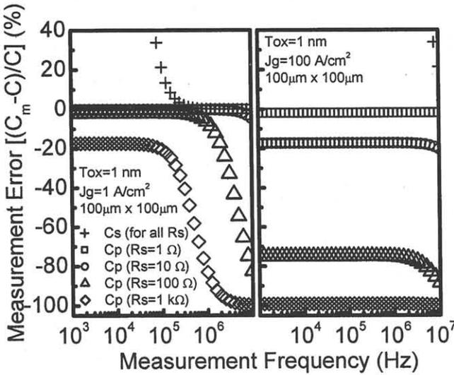
Fig. 3 Systematic error introduced by the coexistence of  $R_s$  and  $R_p$ . As the measurement frequency increases, the impedance of the capacitor decreases. As a result, the impact of  $R_p$  decreases and the impact of  $R_s$  increases. Therefore, the error in series mode, which is independent of  $R_s$ , decreases with frequency while the error in parallel mode increases with frequency. Higher gate leakage is shown on the right.
