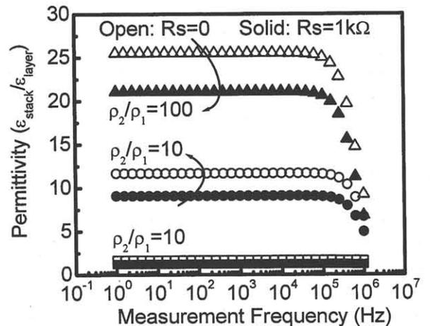
Fig. 6 Dispersion increases as the resistivity ratio  $\rho_1/\rho_2$  increases. Measured dispersion is reduced when  $R_s$  is present. This example assumes both layers have the same permittivity  $\epsilon_{\text{layer}}$ .
