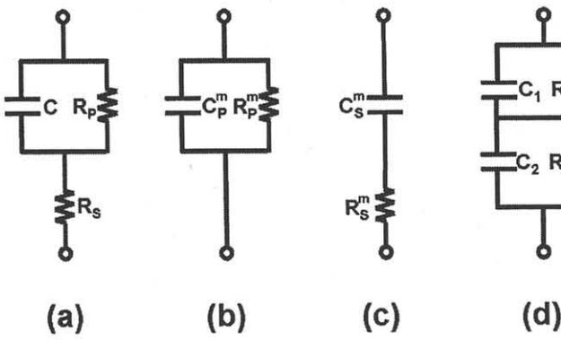
Fig. 1 Small signal circuit representations of MOS capacitors:
