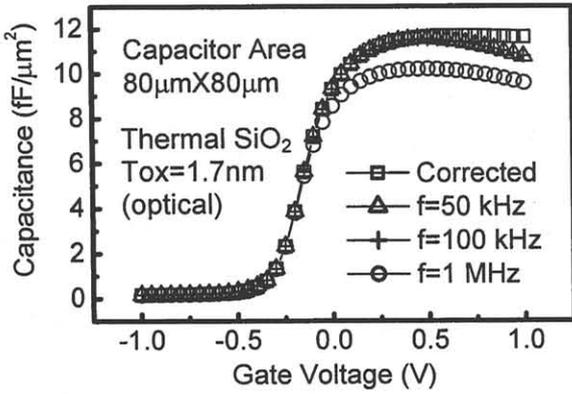
Fig. 2 Measured and corrected high-frequency CV.
