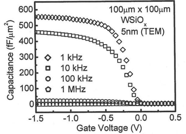
Fig. 5 Three orders of magnitude of dispersion in measured CV.
