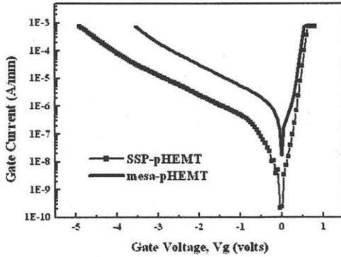
Fig. 2. Schottky diode characteristics of  $\text{Si}_3\text{N}_4$  sidewall planarized PHEMTs (SSP-pHEMT) and conventional mesa-pHEMTs
