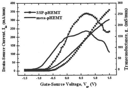
Fig. 3. Device  $g_m$ - $I_{ds}$ - $V_{gs}$  transfer curves characteristics of SSP-pHEMTs and mesa-pHEMTs
