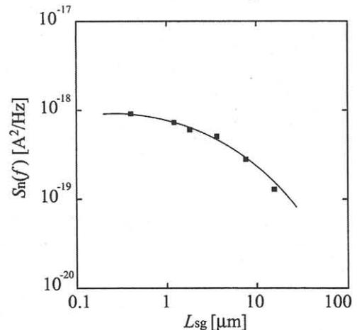
Fig. 5 Noise spectrum densities  $S_n(f)$  at  $V_g - V_{th} = 1.4V$  plotted against  $L_{sg}$ .
