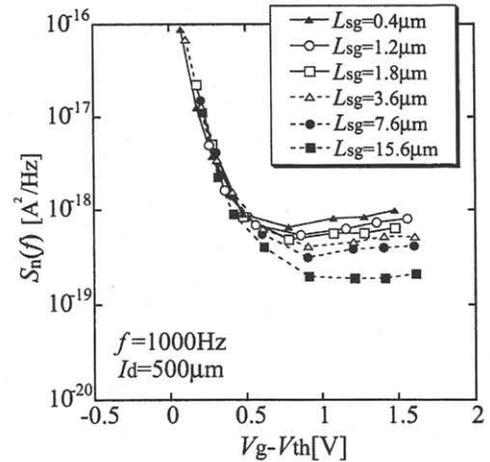
Fig. 4 Dependence of  $S_n(f)$  on  $V_g - V_{th}$  for several devices with different  $L_{sg}$ .
