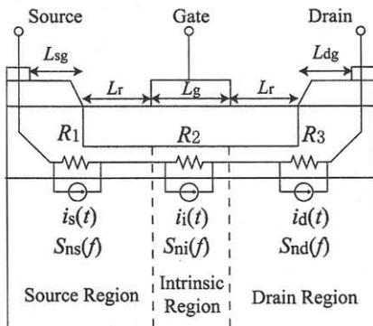
Fig. 2 The noise model used in this study.
