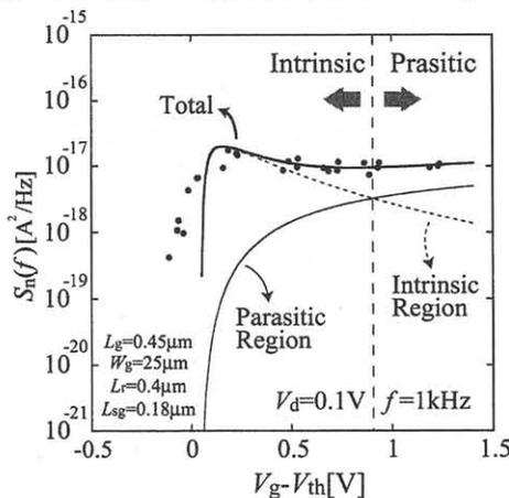
Fig. 3 The contributions of the noise sources located in the intrinsic and parasitic regions to the total LFN.
