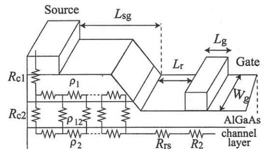
Fig. 6 Transmission Line Model (TLM) proposed by S. J. Lee et al [4]. This model was used in the analysis of LFN generating from the parasitic region.
