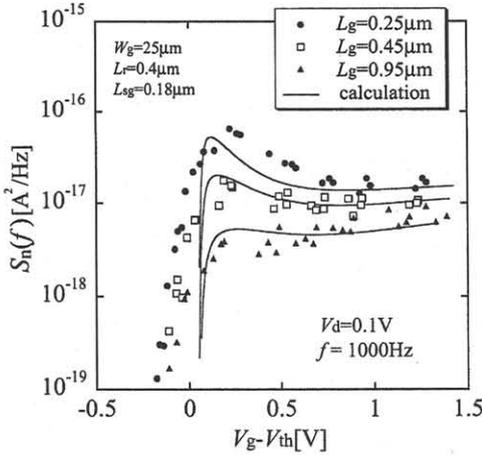
Fig. 1 Noise spectrum densities  $S_n(f)$  at 1000 Hz as a function of  $V_g - V_{th}$  for the devices with different  $L_{sg}$ .
