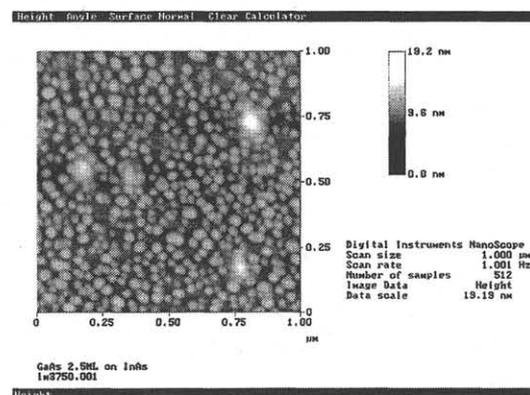
Fig.1 AFM image of 2.5ML GaAs on InAs
