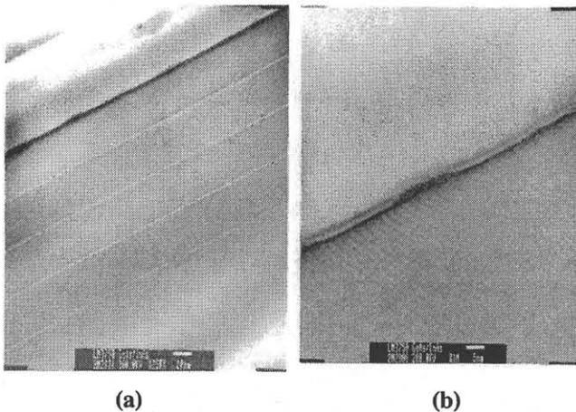
Fig.2 TEM images of 5 layers GaAs (a), and one of GaAs antidots (b).
