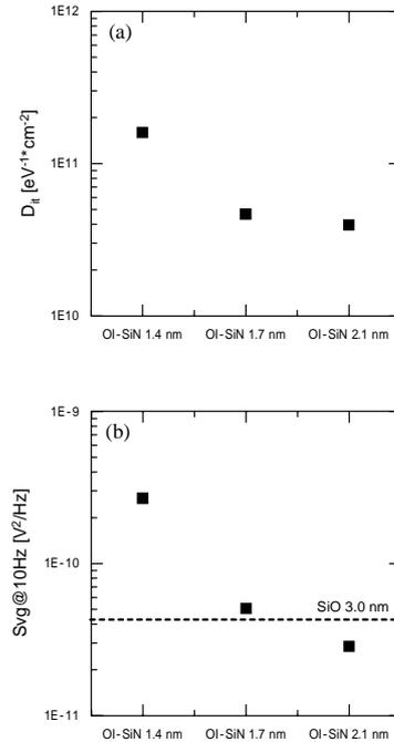
Fig. 5: (a) The interface-state density ( $D_{it}$ ) at mid-gap extracted by charge-pumping method and (b)  $1/f$  noise amplitude at 10 Hz taken from the Fig. 3(a). The dotted line represents the noise level of the device with 3.0-nm  $\text{SiO}_2$  gate dielectric.
