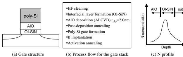
**Fig. 1: AIO/OI-SiN stacked gate device and process flow**
