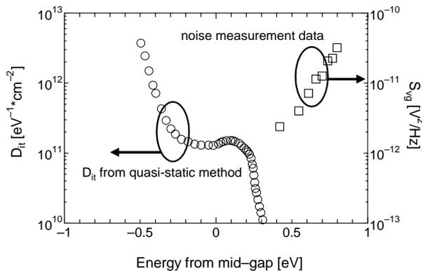
Fig. 4: The dispersion of the interface-state density ( $D_{it}$ ) with interfacial OI-SiN 2.1-nm thick extracted by quasi-static method
