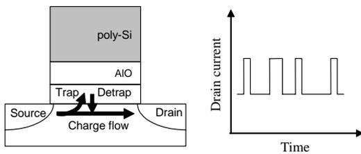
Fig. 3: The mechanism of  $1/f$  noise
