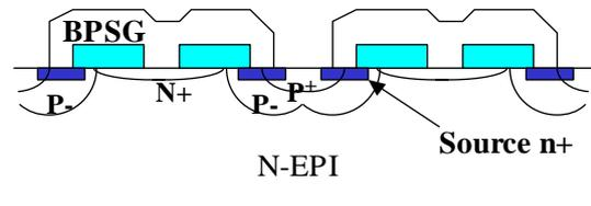
Fig. 1 cross-section of split poly and split p-well structure
