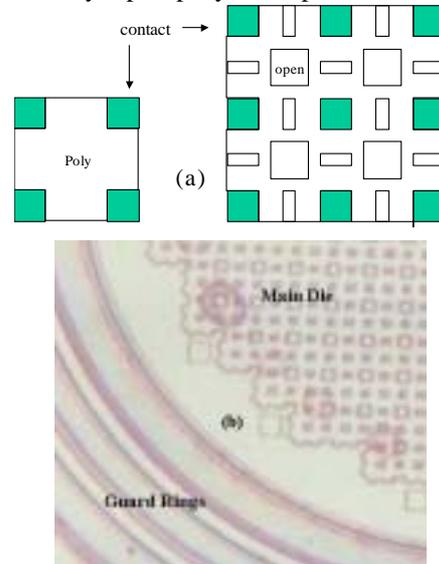
Fig. 2 Top view diagram (a) and photograph (b) of split poly structure
