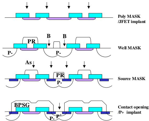
Fig. 3 Process flow of split poly and split p-well device
