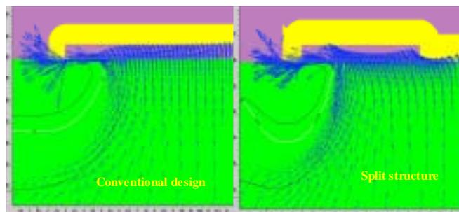
Fig. 5 Simulated current density comparison between conventional and split structure devices
