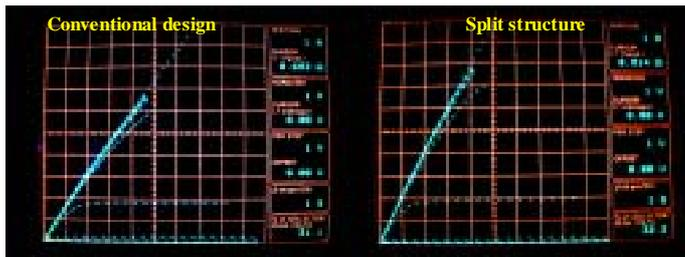
Fig. 4 On state characteristics of conventional and split structure devices
