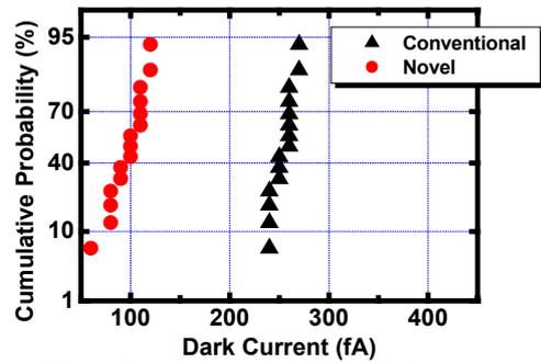
Fig. 5. Cumulative probability of dark current for different photodiode structure.
