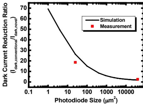
Fig. 6. Dark current cancellation Ratio for photodiode size from 1µm<sup>2</sup> to 40000µm<sup>2</sup>.
