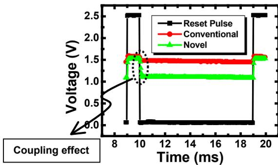
Fig. 3. Illustration of the coupling effect due to the ring-shaped poly-gate.
