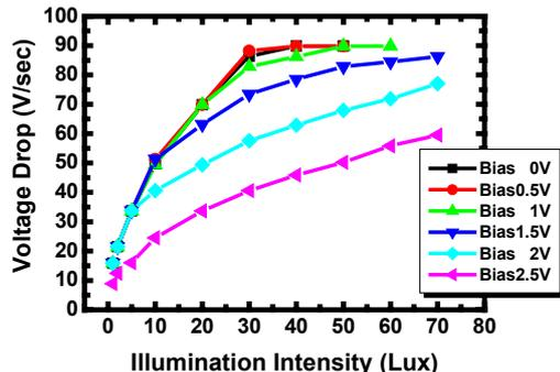
Fig. 9. Dependence of optical sensitivity and dynamic range on bias voltage.
