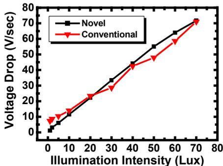
Fig. 8. The optical sensitivity of the novel pixel and the conventional pixel.
