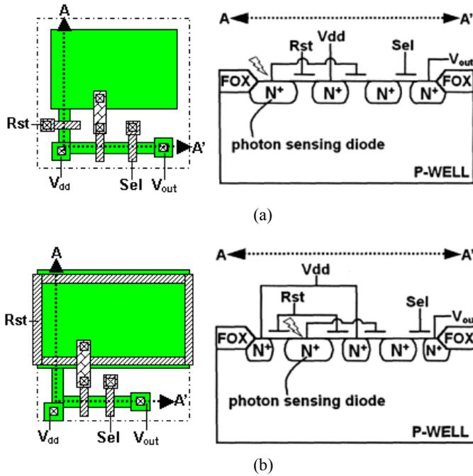
Fig. 1. Layout view and cross-sectional view along-line AA' (a) conventional structure (b) novel structure.
