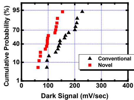
Fig. 7. Cumulative probability of dark signal of the novel pixel and the conventional pixel.
