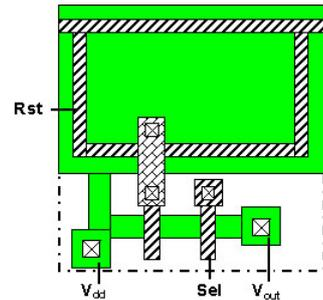
Fig. 2. Novel structure with independent poly-gate ring.
