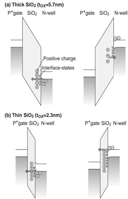
Fig. 5 Schematic diagram of  $V_{TH}$  and Dit degradations under alternate NBT and PBT stress comparing thin and thick  $\text{SiO}_2$  films. In the case of thick  $\text{SiO}_2$ , holes captured in  $\text{SiO}_2$  under NBT stress are released by applying positive bias. Therefore, the recovery of  $V_{TH}$  shift is observed.
