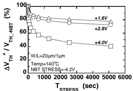
Fig. 3 Recovery ratio of  $V_{TH}$  by applying PBT stress. The recovery ratio is estimated as the ratio of  $V_{TH}$  under NBT stress to that under PBT stress. NBT stress was performed under  $V_G=-4.2 V$  for 5120 sec. It is found that the recovery ratio strongly depends on  $V_G$  of PBT stress.
