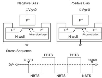
Fig. 1 Schematic diagram of experimental condition. In this work, NBT (in the inversion condition) and PBT (in the accumulation condition) stress were alternately applied.
