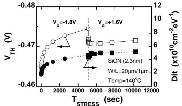
Fig. 6 Threshold voltage shift ( $V_{TH}$ ) and generated interface-state density (Dit) of thin SiON films under NBT and PBT stress. It is found that the recovery of  $V_{TH}$  shift is clearly observed even though oxide thickness is 2.3 nm.
