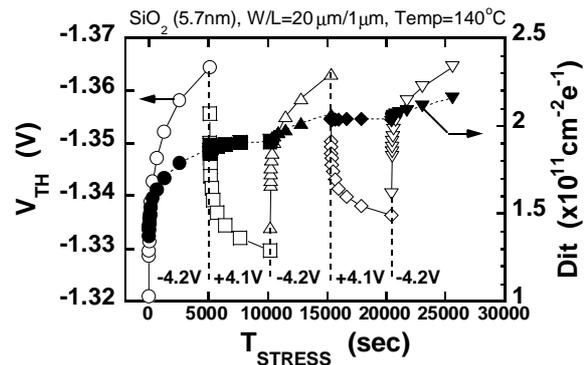
Fig. 2 Threshold voltage shift ( $V_{TH}$ ) and generated interface-state density (Dit) under alternate NBT and PBT stress. Oxide thickness is 2.3 nm. Note that the recovery of  $\Delta V_{TH}$  is observed under PBT stress, though there is no change in Dit during PBT stress.
