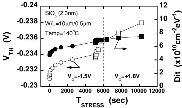
Fig. 4 Threshold voltage shift ( $V_{TH}$ ) and generated interface-state density (Dit) under alternate NBT and PBT stress. Oxide thickness is 2.3 nm. Note that  $V_{TH}$  and Dit monotonically increase even under PBT stress.
