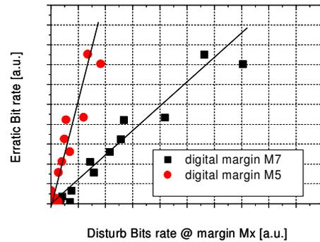
Figure 2: Correlation of Erratic Bit (EB) rate with Disturb Bit (DB) rate, measured at different digital sensing levels Mx
