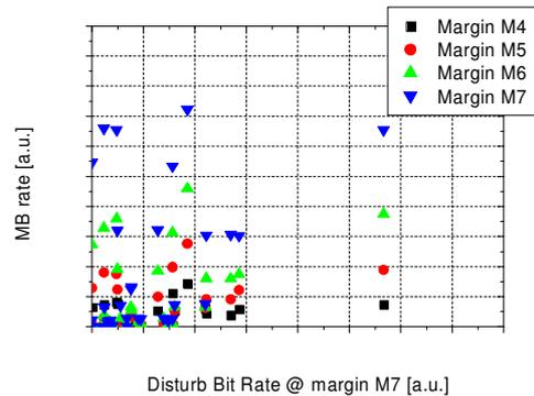
Figure 3: The Moving Bit (MB) rate shows no correlation with Disturb Bit rate independent of sensing level
