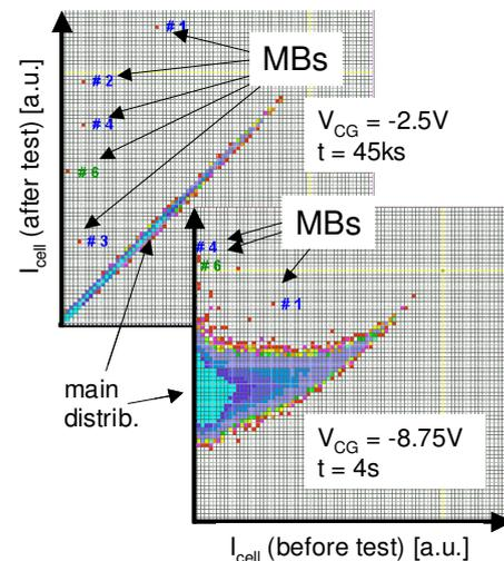
Figure 4: top: analog cell current measurements demonstrate the field acceleration of Moving Bits (MB); bottom: high internal electrical fields generate a lot of additional Disturb Bits etc.
