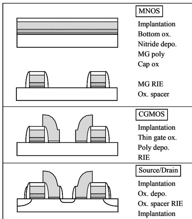
Fig. 2 Cell process sequence
