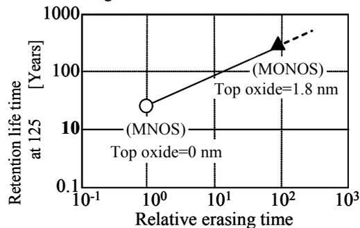
Fig. 7 Trade-off between erasing time and retention life time
