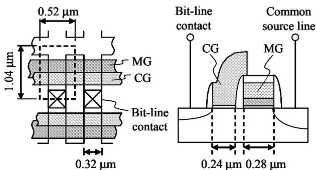
Fig. 1 Cell layout and cross section
