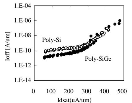
Fig. 11.  $I_{\text{dsat}}$ - $I_{\text{off}}$  characteristics for pFET.  $V_g=V_d=-1.2\text{V}$ .
