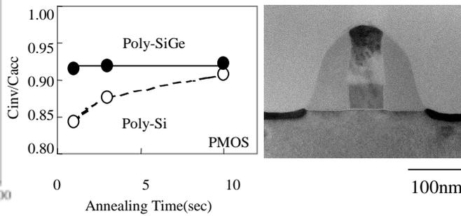
Fig. 6. Annealing-time dependence of B-activation in poly-SiGe and poly-Si. Annealing temperature = 1000°C.
