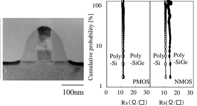
Fig. 7. Cross sectional TEM image of FET using Si/SiGe layered structure with Ni-salicidation.  $L_{\text{gate}}=70\text{nm}$
