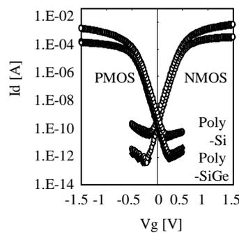
Fig. 10. Subthreshold  $I_d$ - $V_g$  characteristics of n/pFET.  $L/W = 90\text{nm}/10\mu\text{m}$ ,  $V_d=-1.2\text{V}$  and  $-0.05\text{V}$ .
