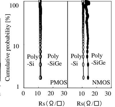
Fig. 8.  $R_s$  distributions of Ni-salicides with the poly-Si and poly-Si/poly-SiGe
