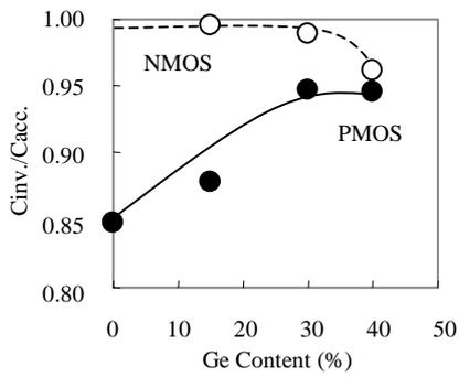
Fig. 1. Ge-content-dependence of the gate-depletion for NMOS and PMOS with 50nm  $\alpha$ -Si/100nm-SiGe deposited at 475°C.
