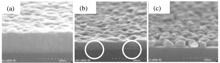
Fig. 2. Thickness dependence of  $\text{Si}_{0.7}\text{Ge}_{0.3}$ -film morphology. Thickness of (a), (b), and (c) are 150nm, 50nm, and 20nm.
