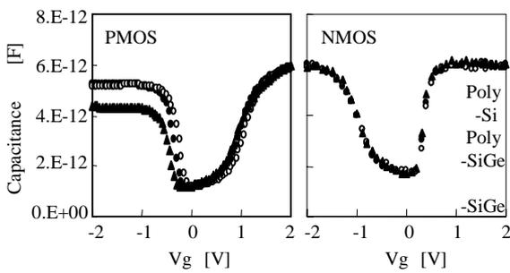
Fig. 9. C-V characteristics for P- and N-capacitor. Area=400 $\mu\text{m}^2$ .
