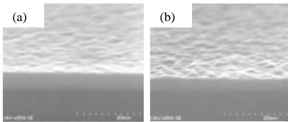
Fig. 3. Pressure dependence of  $\text{Si}_{0.7}\text{Ge}_{0.3}$ -film morphology. (a) 200Pa, (b) 10Pa. Thickness is 50nm.
