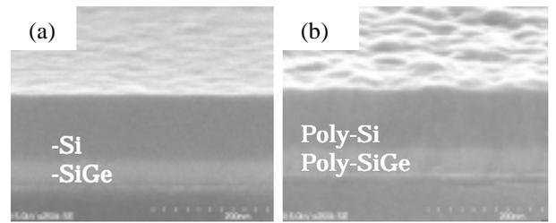
Fig. 4. Si/ $\text{Si}_{0.7}\text{Ge}_{0.3}$  layered structure for salicidation. (a) -SiGe followed by -Si deposition at 530°C. (b) Poly-SiGe followed by Poly-Si deposition at 620°C.
