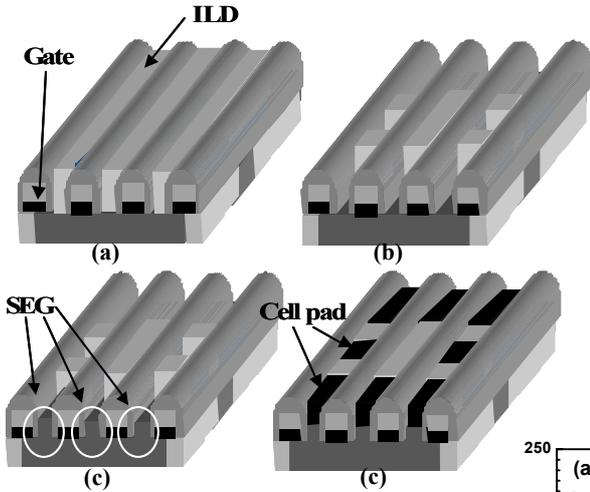
Fig. 3. Schematic diagrams for the SAC-SEG process flow. (a) the first ILD layer was deposited, (b) cell contacts were opened by SAC etch, (c) after the SEG, (d) cell pad poly was deposited. Bridges between the storage nodes can be prohibited by the ILD layers in the SAC-SEG process.
