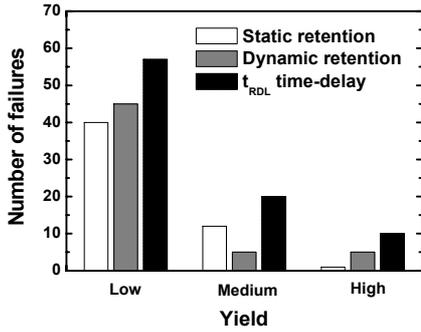
Fig. 1. Trends of the number of failures for three major failure modes of the recent DRAM product. The  $t_{RDL}$  which directly depends on the  $I_{DSAT}$  is a dominant factor.
