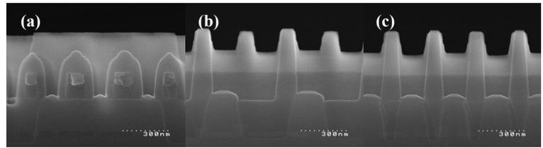
Fig. 4. Cross-sectional SEM images for the DRAM cells. (a) cross-section cut along the bit-line direction (A-A'), (b) along the word-line direction through direct contacts (DC)(B-B'), (c) word-line direction through storage nodes (C-C'). The right hand side drawing shows active and word-lines.
