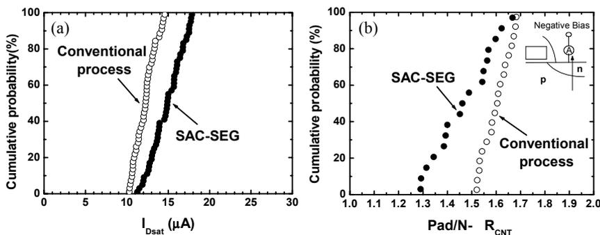
Fig. 6. Saturation current and contact resistance distributions. (a) saturation current distribution, (b) contact resistance distribution. The figures clearly show that the  $I_{DSAT}$  increase for the SAC-SEG was originated from the  $R_{CNT}$  reduction.
