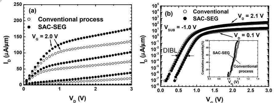
Fig. 5. Saturation current and sub-threshold characteristics for the cell transistors fabricated using the conventional process (without SEG) and the SAC-SEG process. (a) saturation current characteristics. (b) sub-threshold characteristics. Insertion: distribution of the threshold voltages for the two samples.
