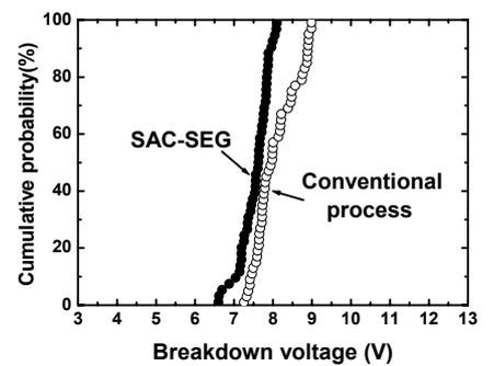
Fig. 7. Breakdown voltage distribution, drain voltages for 10nA source-to-drain leakage current at the off-state, for the SAC-SEG and conventional process.
