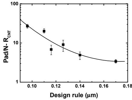
Fig. 2. Contact resistance for the DRAM cell contacts as a function of the design-rule.
